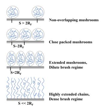
Figure 3. Conformation and layer structure oftethered polymer chains.  $R_F$  is the Flory radius of the chains.
