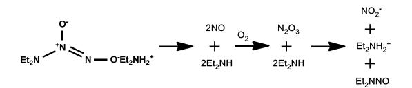
Handa et al<sup>197</sup> investigated PVC modified by incorporation of diazeniumdiolated dibutylhexanediamine. They showed that the rate of NO release from modified catheters into a buffer solution was in the physiologic range and was sustained over periods of several days. The patency rate of arteriovenous shunts in rabbits was greater for the modified materials compared to controls.
