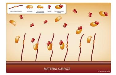
Figure 6. CBAS end point attachment of heparin. Adapted with permission from Carmeda AB.
