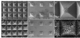
Figure 6 SEM images: top view of calcium sulfate (CaS) microneedles (MNs) after release tests: densely arranged (a), sparsely arranged (b), and highly magnified densely arranged needles (c); top view of calcium phosphate (CaP) microneedles (MNs) after release tests: densely arranged as (d), sparsely arranged (e), and highly magnified densely arranged needles
