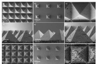
Figure 4 SEM images: top view of intact calcium sulfate (CaS) microneedles (MNs): densely arranged (a), sparsely arranged (b), and highly magnified densely arranged needles (c); cross-section view of CaS
