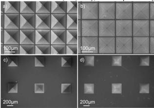
Figure 2 master mold (a and c) and positive replicate (b and d)
