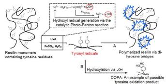
**Fig. 3** Mechanism of resilin cross-linking via the photo-Fenton reaction. Hydrogen abstraction from tyrosine via strong oxidizing agent (.-OH) can generate tyrosyl radical, resulting in di-tyrosine bridges (A) and other tyrosine oxidation products (B). (Reproduced with permission from ref. 24, Elsevier, Copyright 2011).
