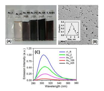
**Fig. 7** (A) Optical micrograph of AuNPs-rec1-resilin nanobioconjugates exhibiting surface plasmon resonance at different Au cation:rec1-resilin molar ratios. (B) TEM images of rec1-resilin capped gold nanoparticles synthesized at Au cation:rec1-resilin molar ratio of 2.12. (C) Fluorescence emission spectrum from the aqueous sols of rec1-resilin protected AuNPs (sample designations per Table 2). (Reproduced with permission from ref. 61, Elsevier, Copyright 2011).
