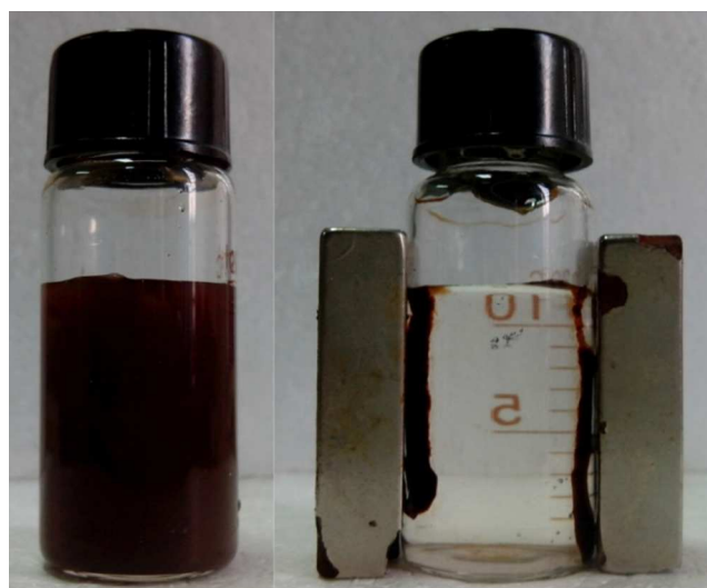
Fig.3 MCNCs-5 (left) dispersed in aqueous solution and MCNCs-5 attracted by external magnetic fields (right).
