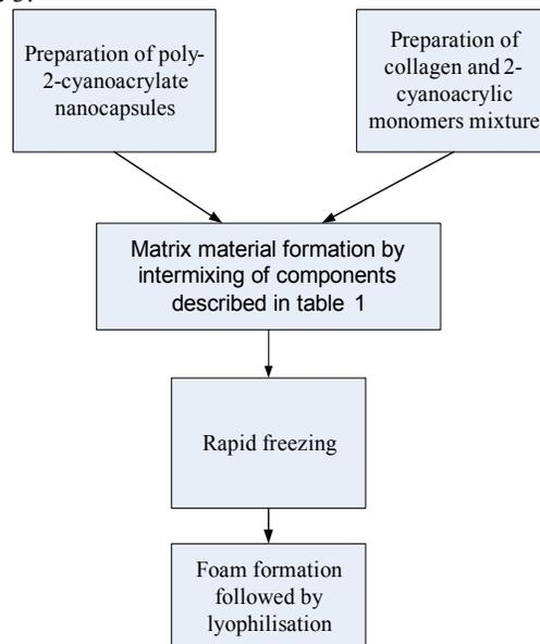
Scheme 4. Block-scheme of porous implant preparation. Initial composition contains three components: the matrix material, insulin containing nanocapsules and polymerization medium. Then it was frozen with formation of solid block giving foam after water evaporation by lyophilisation. As
