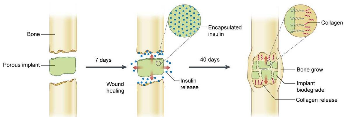
It has been developed a novel polycyanoacrylate based bone substituting foam material providing independent release of two polypeptide actives with followed biodegradation and bone substitution.
