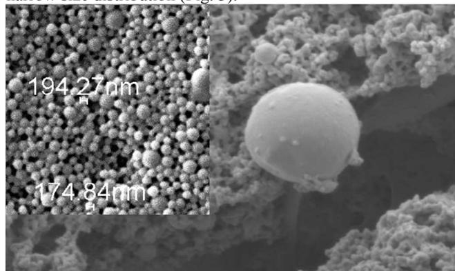
Figure 3. SEM image of poly-2-cyanoacrylate nanocapsules. Isolation of capsules comprises stage of lyophilisation followed by washing out components of polymerization medium. The freezing results partial insulin inactivation, however not less than 25% of its initial activity still remains. It is much more than enough to provide the material with wound healing properties.
