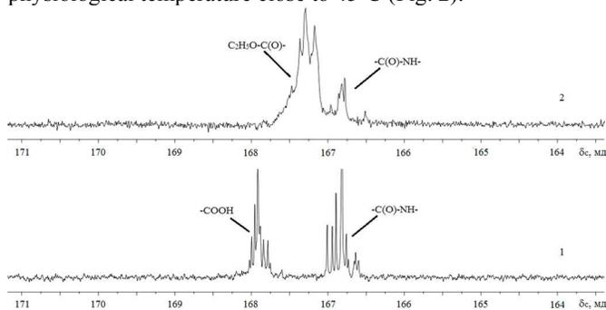
Figure 2. Fragment of  $^{13}\text{C}$  NMR spectra of poly-2-cyanoacrylic acid (1) and 2-cyanoacrylic acid/ethyl-2-cyanoacrylate copolymer (2)
