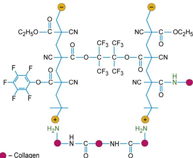
Figure 1. Key steps of copolymer chemical modification. Introduction of collagen into the material significantly drops mechanical properties of the foam and increases rate of its biodegradation. Actually 30% additive is a maximum which keeps acceptable compression strength.
