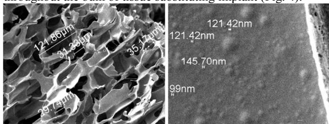
Figure 4. SEM image of porous material (left) and nanocapsules incorporated into its wall (right)
