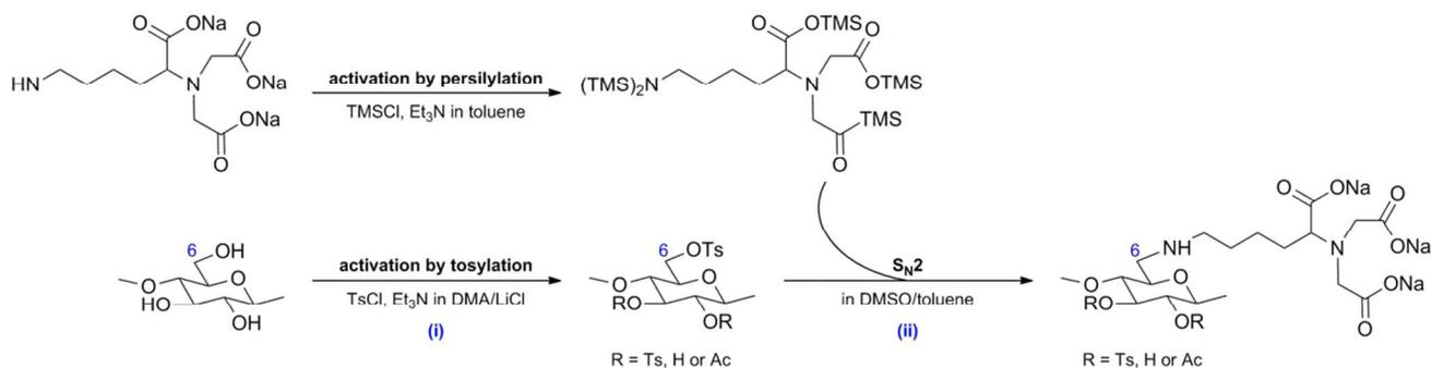
Figure 11 Synthesis of nitrilotriacetic acid (NTA)-modified amino-cellulose.
