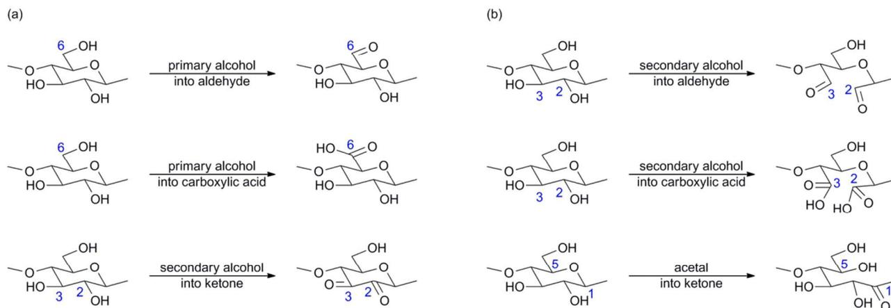
**Figure 10** Main oxidation reactions of cellulose (a) without ring opening and (b), with ring opening.
