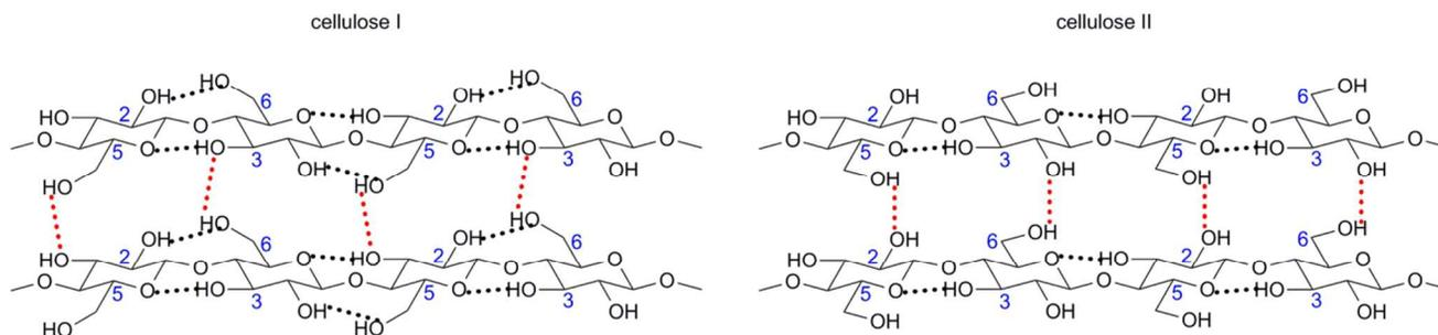
**Figure 5** Supramolecular distinction between cellulose I and cellulose II lies in inter- and intramolecular hydrogen bonds.
