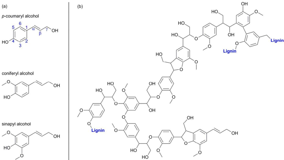
Figure 8 (a) The three monomers of lignin. (b) A representative fragment of lignin structure.
