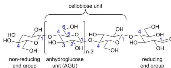
**Figure 1** Cellulose molecular structure ( $n=DP$ , degree of polymerization).
