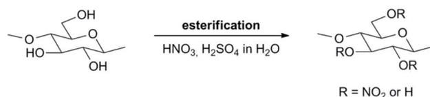
Figure 12 Esterification of cellulose into nitrocellulose.
