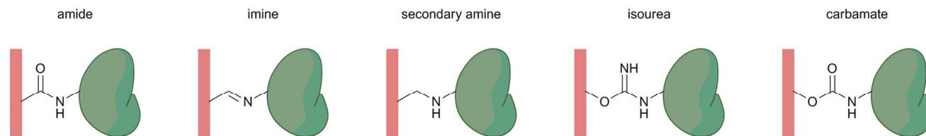
**Figure 20** Nature of the linking bonds between cellulose substrate and biomolecules.
