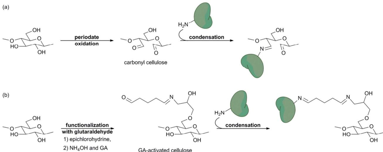
**Figure 22** Imine bond formation (a) through periodate oxidation of cellulose and (b) through functionalization with glutaraldehyde.
