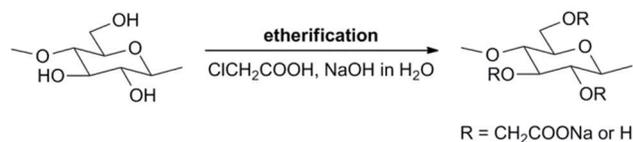
Figure 13 Etherification of cellulose into carboxymethyl cellulose.
