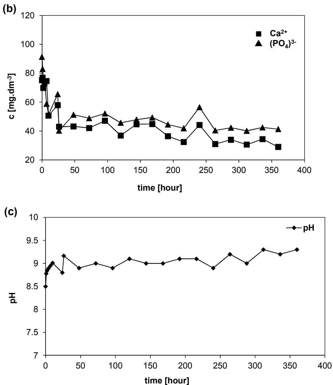
**Fig. 4.** Concentrations of (a) Si, (b)  $\text{Ca}^{2+}$ ,  $(\text{PO}_4)^{3-}$  ions and (c) values of pH in I-solution during interaction with scaffolds
