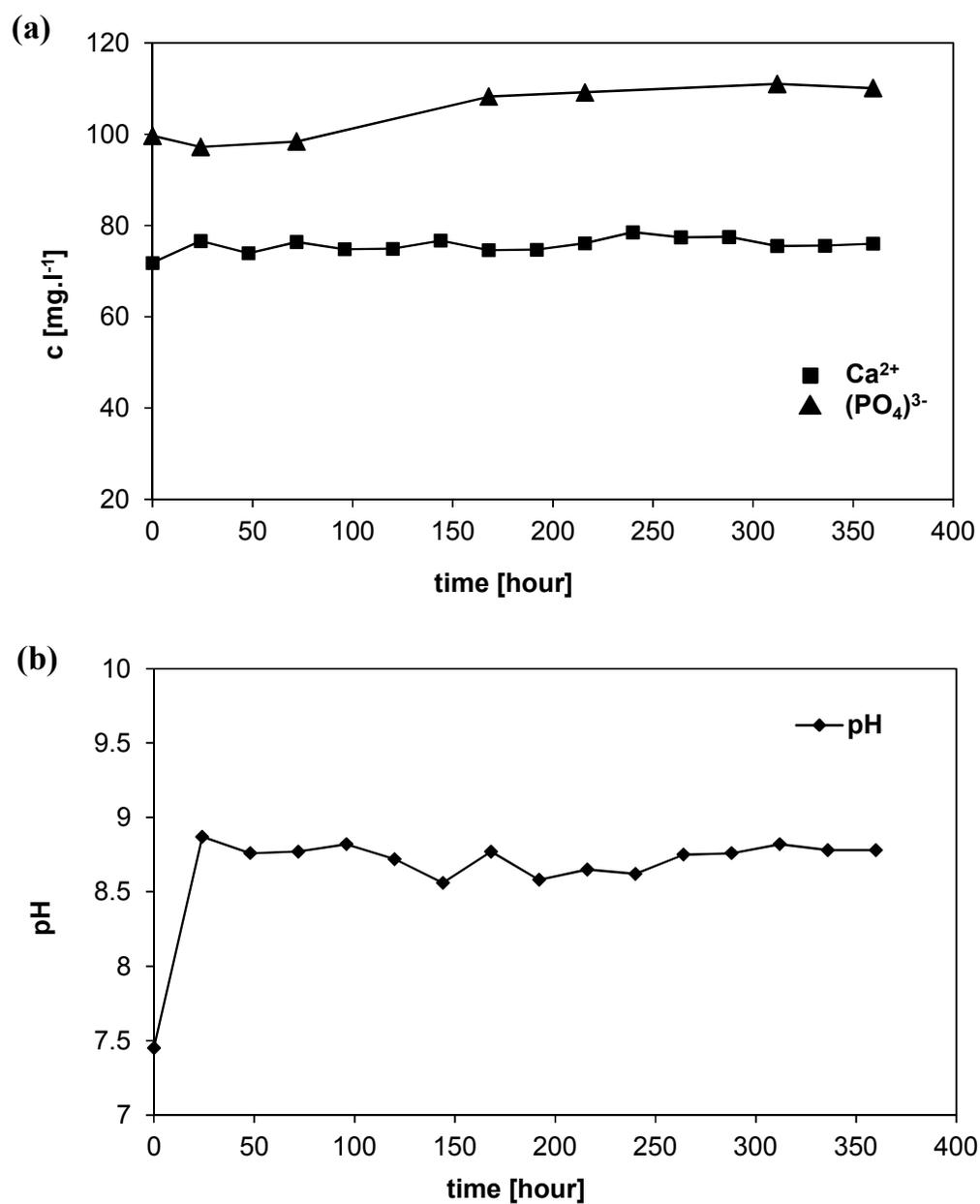
**Fig. 1.** Concentrations of (a)  $\text{Ca}^{2+}$ ,  $(\text{PO}_4)^{3-}$  ions and (b) values of pH in mod-DMEM during interaction with scaffolds
