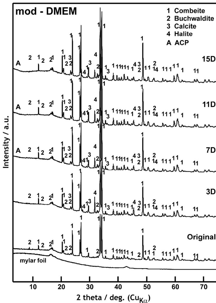
**Fig. 2.** XRD patterns of scaffold before and after 3, 7, 11 and 15 days of interaction with mod-DMEM
