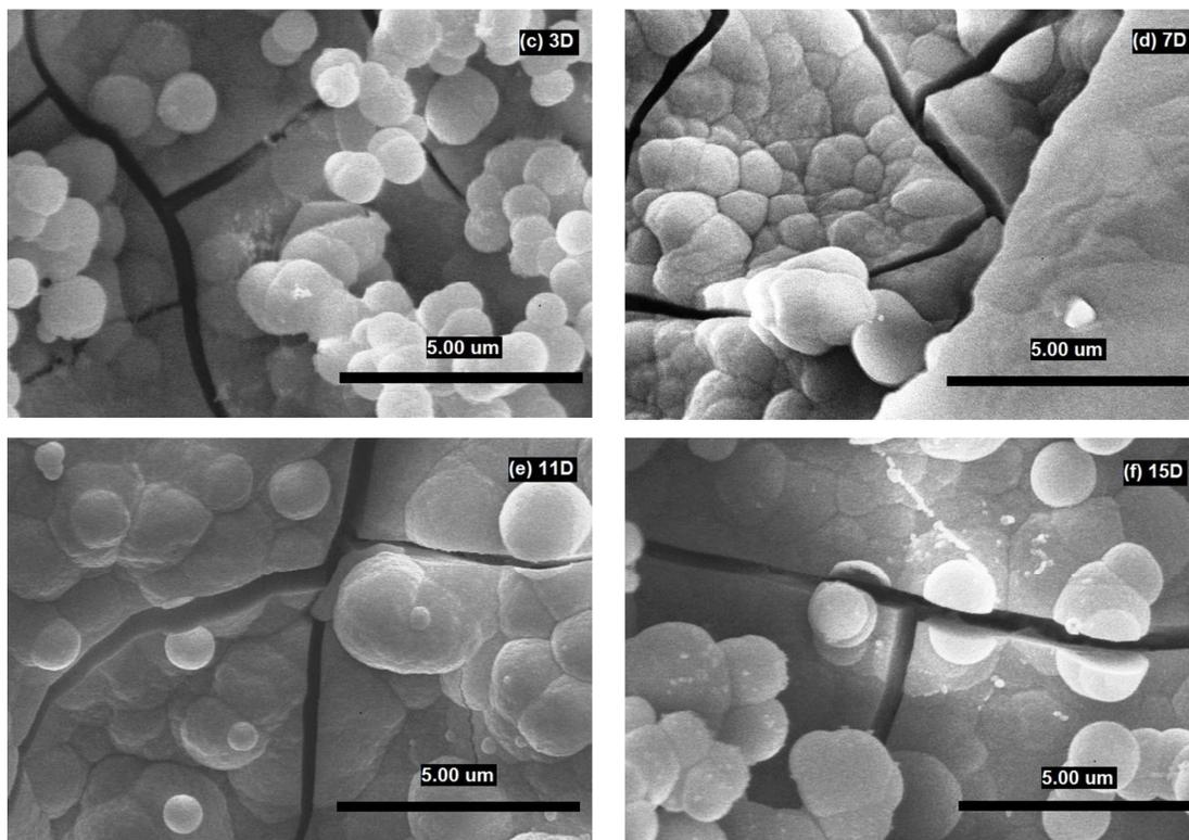
**Fig. 6.** SEM images of scaffolds (a) before (combeite - the small tabular crystals, buchwaldite and structurally isomorphic phase  $\text{CaO}\cdot\text{SiO}_2$  - needle-like crystals) and after (b) 1, (c) 3, (d) 7, (e) 11 and (f) 15 days of interaction with I-solution. The fractures in the newly developed layers were caused by drying of samples.
