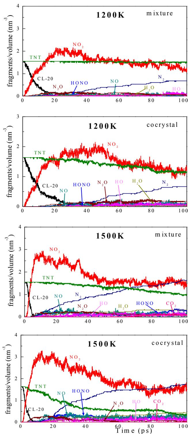
**Figure 16.** Evolution of intermediate and secondary products of the mixture and cocystal systems from NVT MD simulations.
