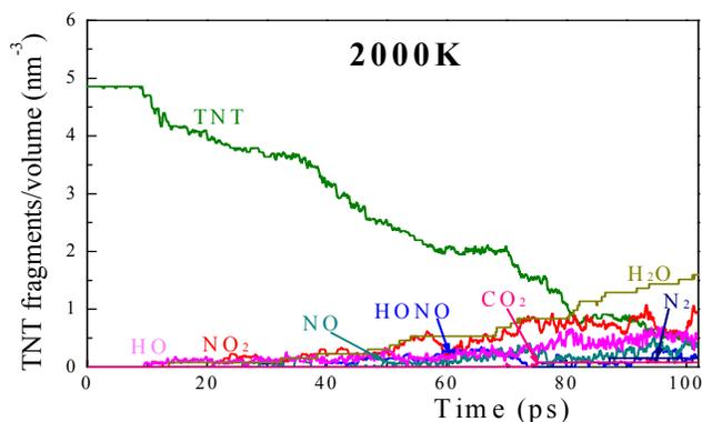
**Figure 8.** Time evolution of chemical products of TNT under 2000K. The slow dissociation rate indicates that TNT has a different decomposition mechanism than CL-20.
