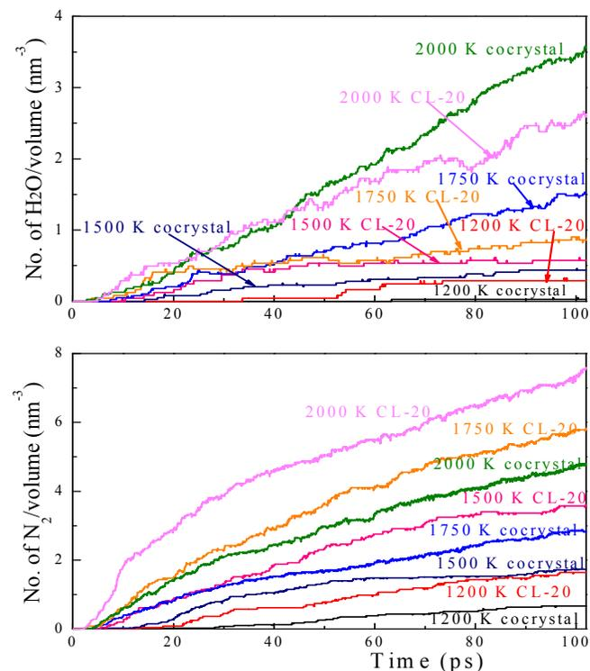
**Figure 7.** The number of final products  $\text{H}_2\text{O}$  and  $\text{N}_2$  fragments during MD-NVT simulations. These final products were produced earlier in CL-20 than the cocystal during the decomposition process, indicating more intense chemical reactions in CL-20 system.
