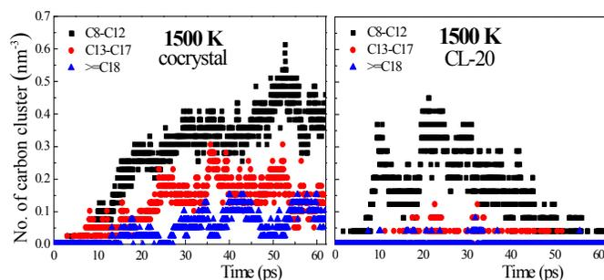
**Figure 13.** Time evolution of three types of carbon cluster formed during NVE-MD for cocrystal and CL-20
