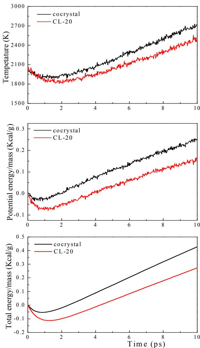
**Figure 10.** Time evolution of temperature, potential energy, and total energy for 10 ps variable-volume MD simulations.
