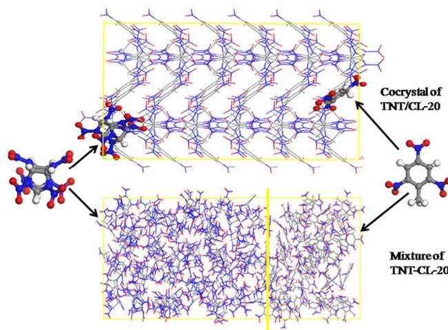
**Figure 2.** Comparison of the TNT/CL-20 cocrystal structures and the TNT-CL-20 mixture. The mixture is made by combining a slab of amorphous TNT with a slab of CL-20 molecules each separately into one half side of the supercell, whereas the cocrystal has an ordered sandwich structure.**Table 3.** The lattice parameters and density ( $\rho$ ) of the cocrystal of TNT/CL-20, compared to the mixture system
