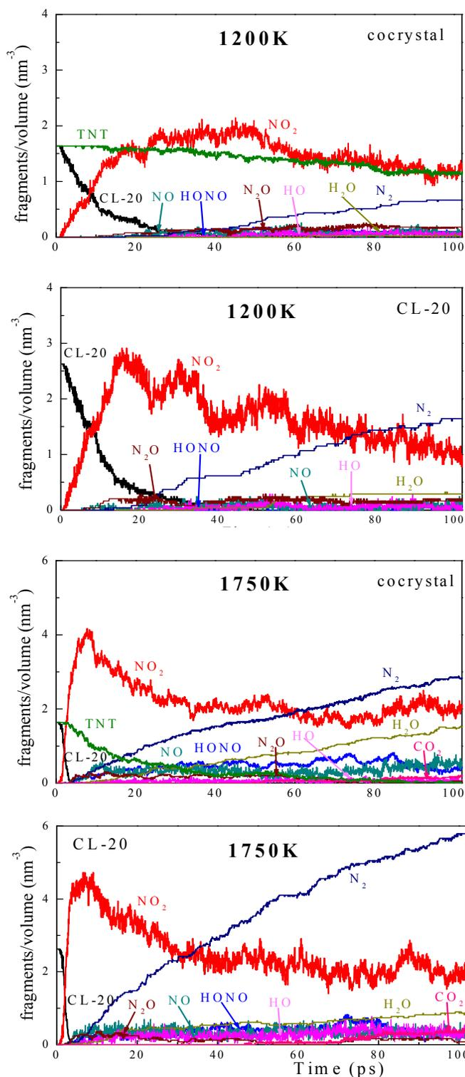
**Figure 6.** Evolution of intermediate and secondary products of cocystal and CL-20 during NVT MD simulation. Chemical reactions occur more intensely in CL-20 than in the cocystal at each
