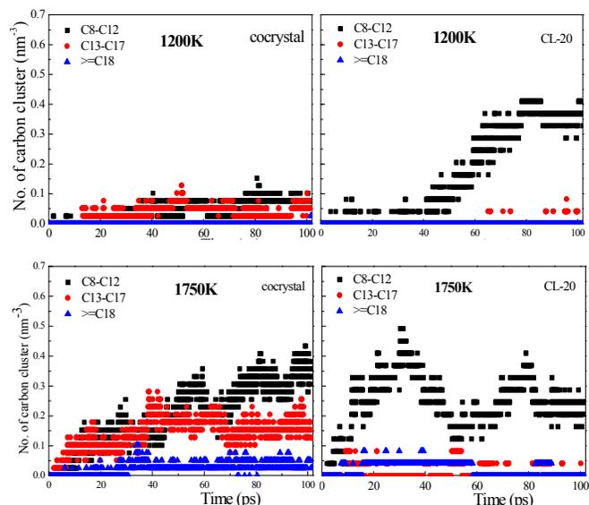
**Figure 9.** Time evolution of three types of carbon cluster formed during decomposition for cocrystal and CL-20. More and bigger carbon-rich aggregates are observed in the cocrystal than for CL-20, leading to a slower chemical reaction process.
