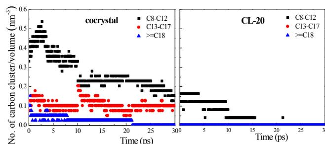
**Figure 11.** Time evaluation of three types of carbon clusters during expansion and the next NVE simulations
