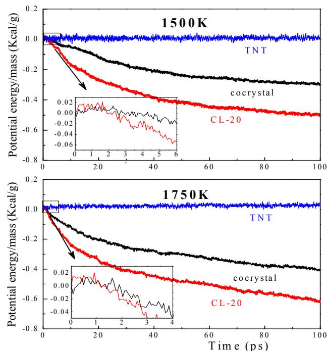
**Figure 3.** Evolution of potential energy in the NVT MD simulations of CL-20, cocrystal and TNT. The initial potential energy is set to zero as a reference. For CL-20 and the cocrystal, the rate of potential energy decrease depends strongly on the temperature, whereas TNT does not react significantly under the conditions studied here. At each temperature, the energy release rate of CL-20 is faster than that of cocrystal, which is much faster than TNT.
