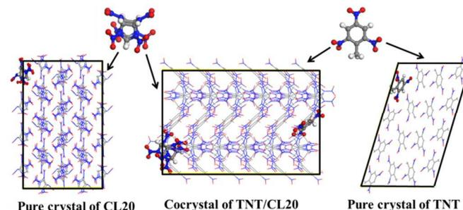
**Figure 1.** Structures of the CL-20 and TNT molecules and structures of the CL-20 crystal, TNT/CL-20 cocrystal, and TNT crystal. The cocrystal, composed of a 1:1 molar ratio of molecules CL-20 and TNT, leads to a sandwich structure of CL-20 molecule layers separated by TNT ones.
