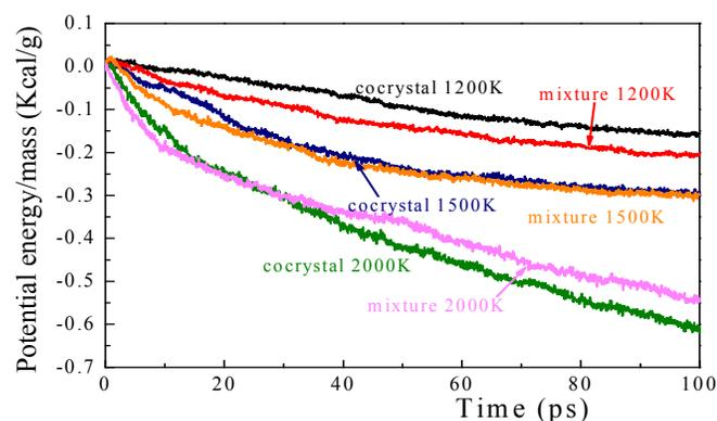
**Figure 14.** Evolution of potential energy in MD-NVT simulations of cocrystal and CL-20/TNT mixed system.
