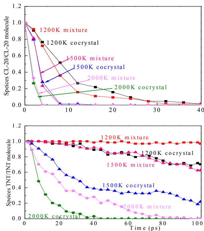
**Figure 15.** The number of remaining CL-20 and TNT and dissociated  $\text{NO}_2$  molecules during MD-NVT simulations.
