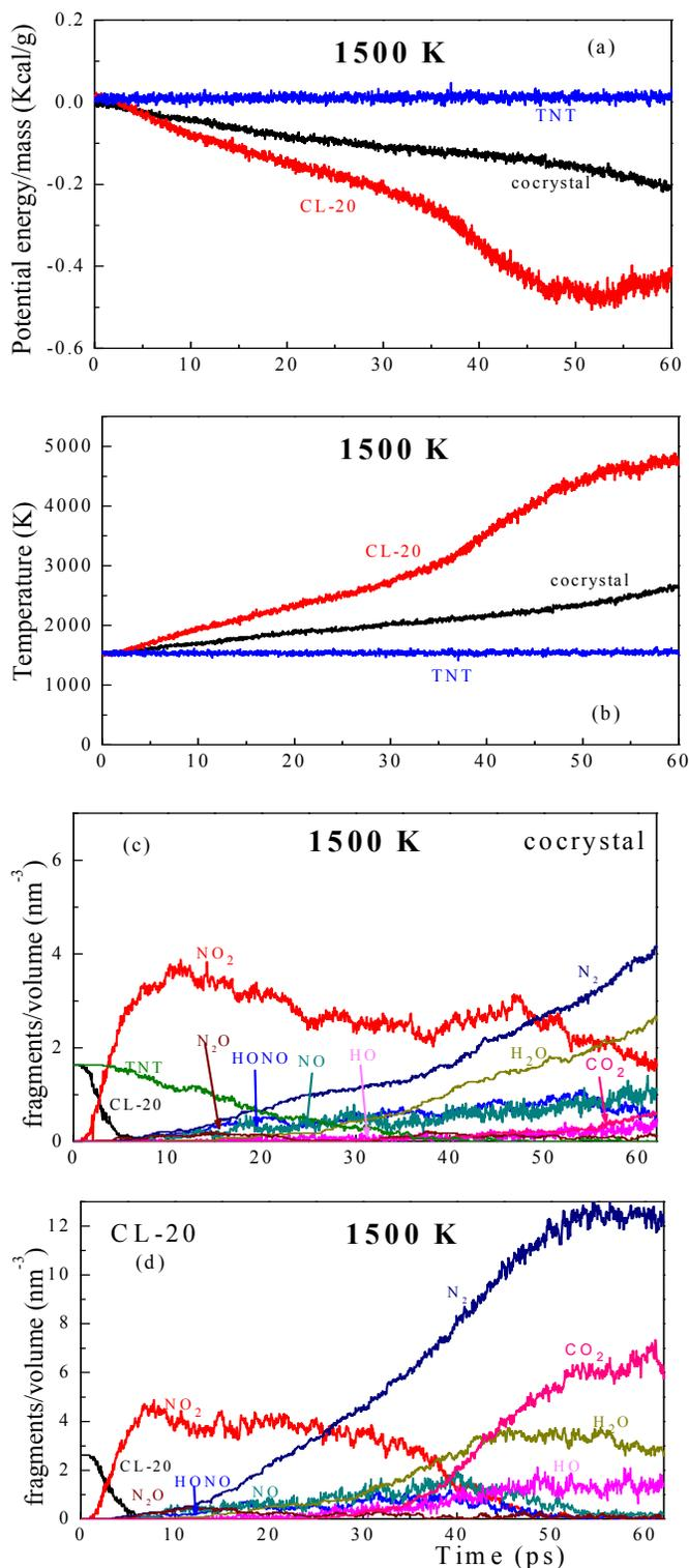
**Figure 12.** Normalized potential energy and temperature as a function of time in the NVE MD with an initial temperature  $T = 1500\text{K}$ . The initial potential energy is set to zero as a reference.
