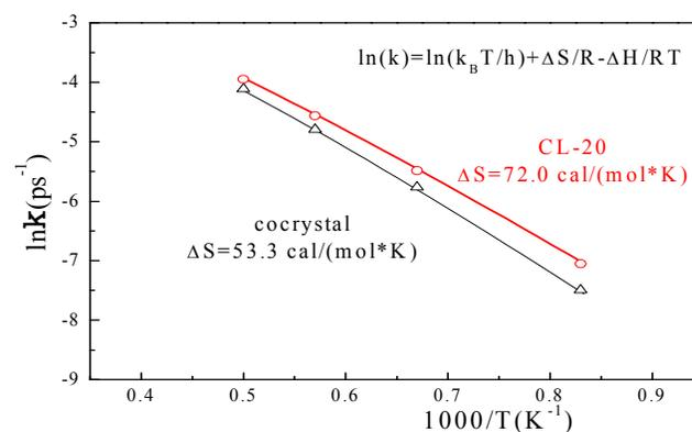
**Figure 4.** Reaction rates for cocrystal TNT/CL-20 and pure crystal CL-20 vs inverse temperature ( $1000/T$ ). The calculated effective activation entropy of chemical reactions is 53.3 cal/(mol\*K) for cocrystal and 72.0 cal/(mol\*K) for CL-20.
