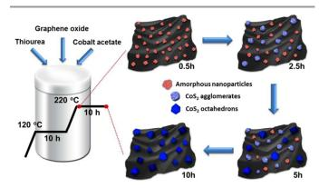
**Figure 5.** Proposed growth schematic of CoS<sub>2</sub> octahedron nanoparticles supported on nitrogen and sulfur doped graphene.
