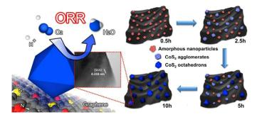
Shape controlled cobalt disulfide octahedron nanoparticles are grown on nitrogen/sulfur-doped carbon nanotubegraphene composites as active non-precious oxygen reduction catalysts.
