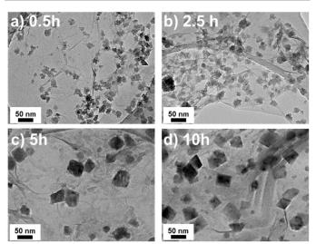
Figure 4. TEM images of the time dependent growth of  $CoS_2$  supported on graphene held at 220  $^\circ C$  for (a) 0.5 h, (b) 2.5 h, (c) 5 h and (d) 10 h.
