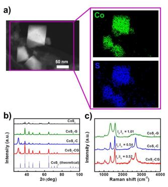
Figure 2. (a) EDX colour mapping of CoS2-CG, (b) XRD patterns of prepared samples and theoretical CoS2 pattern, and (c) Raman spectra for CoS2-G, CoS2-C and CoS2-CG.
