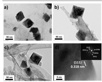
Figure 1. TEM images of (a)  $CoS_2$ -G, (b)  $CoS_2$ -C and (c)  $CoS_2$ -CG. (d) High resolution TEM image of a single crystal  $CoS_2$  octahedron particle along with (inset) SAED pattern.
