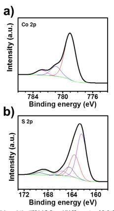
Figure 3. High resolution XPS (a) Co2p and (b) S2p spectra of CoS<sub>2</sub>-CG.
