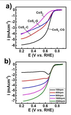
Figure 6. ORR polarization curves (a) at 1600 rpm for all samples, and (b) at various electrode rotation rates for  $CoS_2$ -CG.
