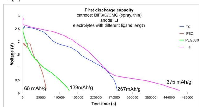
**Fig. 6** Discharge capacities versus electrolyte. Comparison of the first discharge capacities of cells using electrolytes of different lengths with  $\text{BiF}_3/\text{CMC}/\text{C}$  cathodes and lithium anodes (the capacities are not constant and can easily show variation of  $\pm 50 \text{ mAh/g}$ , typical discharge curve and capacities were chosen for this figure).
