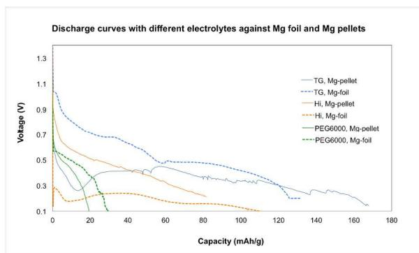
**Fig. 7** Discharge capacities versus anode configuration. Discharge performance with Mg pellet or foil anodes as a function of electrolyte (the capacities are not constant and can easily show variation of  $\pm 30 \text{ mAh/g}$ , typical discharge curve and capacities were chosen for this figure).
