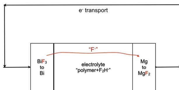
Fig. 1 Fluoride-ion battery configuration. Discharge process for the BiF<sub>3</sub> cathode and Mg anode system.
