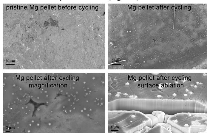
**Fig. 8** SEM images of anodes. Before and after SEM images of Mg anodes after battery discharge tests. Mg pellets pristine (upper left photo), and after cycling (upper right photo). With magnification of the particles (lower left photo) and with surface ablation (lower right photo)
