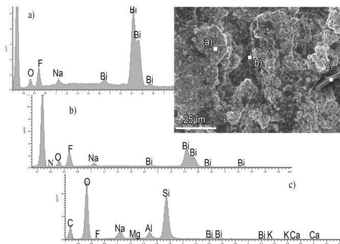
**Fig 12.** EDX measurement of the surface of a discharge  $\text{BiF}_3$ -cathodes, at different places
