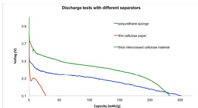
**Fig 13.** Discharge curves of  $\text{BiF}_3$  against Mg with three different separators
