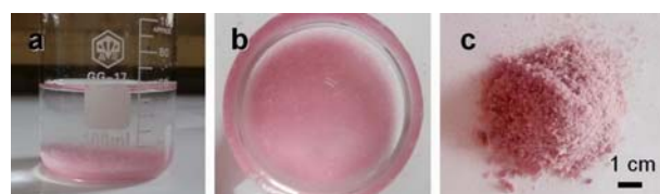
Fig. 1 Schematic illustration of the hydrothermal synthesis of the CQU-Chen-OA-Co-1-1 and corresponding digital photography of the samples (a) and (b) in 100 ml beaker after hydrothermal reaction and (c) after freeze-drying.
