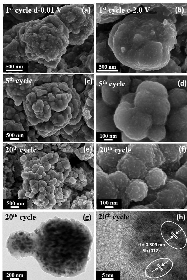
Figure 4 Morphological evolution of the Sb@C microspheres upon fully discharged to 0.01 V and charged to 2.0 V. a) and b) SEM images after the 1 st discharge and charge. c) and d) SEM images after the 5 th discharge and charge. e) and f) SEM images after the 20 th discharge and charge. TEM image g) and high resolution TEM image h) after the 20 th charge.
