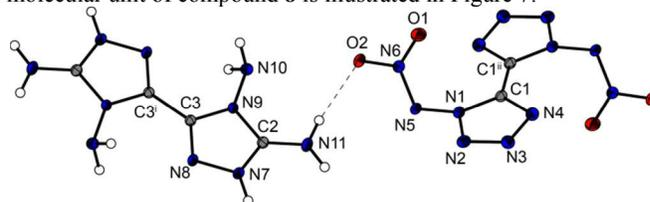
**Figure 7.** Molecular unit of **8**. Ellipsoids are drawn at the 50% probability level. Selected bond lengths [Å]: C1–C1<sup>i</sup> 1.443(3), C3–C3<sup>i</sup> 1.448(2), C2–N11 1.317(2); selected torsion angles [°]: N4–C1–C1<sup>i</sup>–N1<sup>i</sup> 1.7(3), N8–C3–C3<sup>i</sup>–N9<sup>i</sup> 0.2(2); symmetry code: (i) 2–x, 1–y, –z (ii) –x, –y, 2–z.
