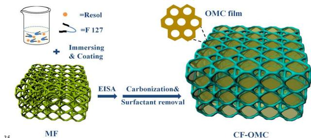
Figure 1. Scheme for preparation of CF-OMC.
