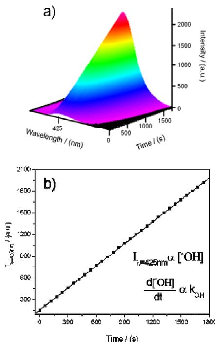
**Figure 5.** PL response of 2-hydroxyterephthalic acid excited at 315 nm. a) Spectra obtained each 60 s with continuous UV irradiation. b) Plot of the maximum intensity against irradiation time. The slope of the curve is directly proportional to TiO<sub>2</sub>-SnO<sub>2</sub> interface formation.
