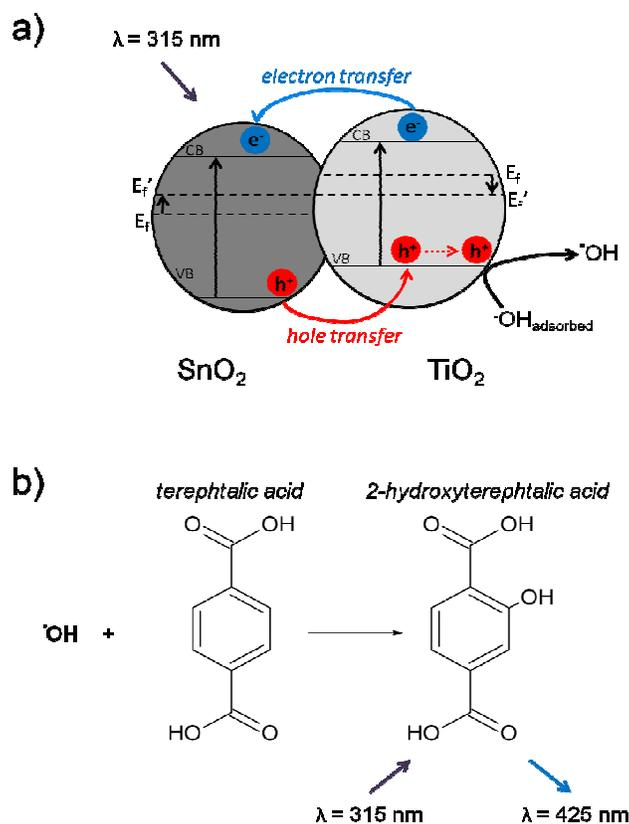
**Figure 4.** a) Band alignment of type-II  $\text{TiO}_2\text{-SnO}_2$  heterostructure and formation of hydroxyl radicals. b) The as-formed hydroxyl radical group is detected by the fluorescence response of 2-hydroxyterephthalic acid at  $\lambda=425$  nm, excited with the same radiation used for oxide excitation ( $\lambda=315$  nm).
