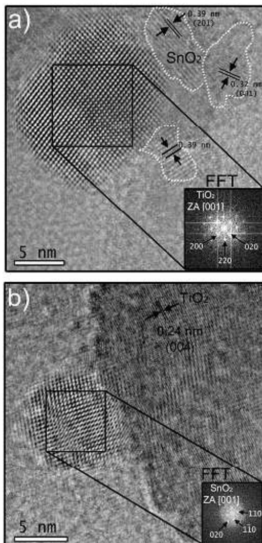
**Figure 3.** High-resolution transmission electron microscopy images for samples containing 20 wt. % SnO<sub>2</sub> hydrothermally treated at a) 150 °C and b) 175 °C.
