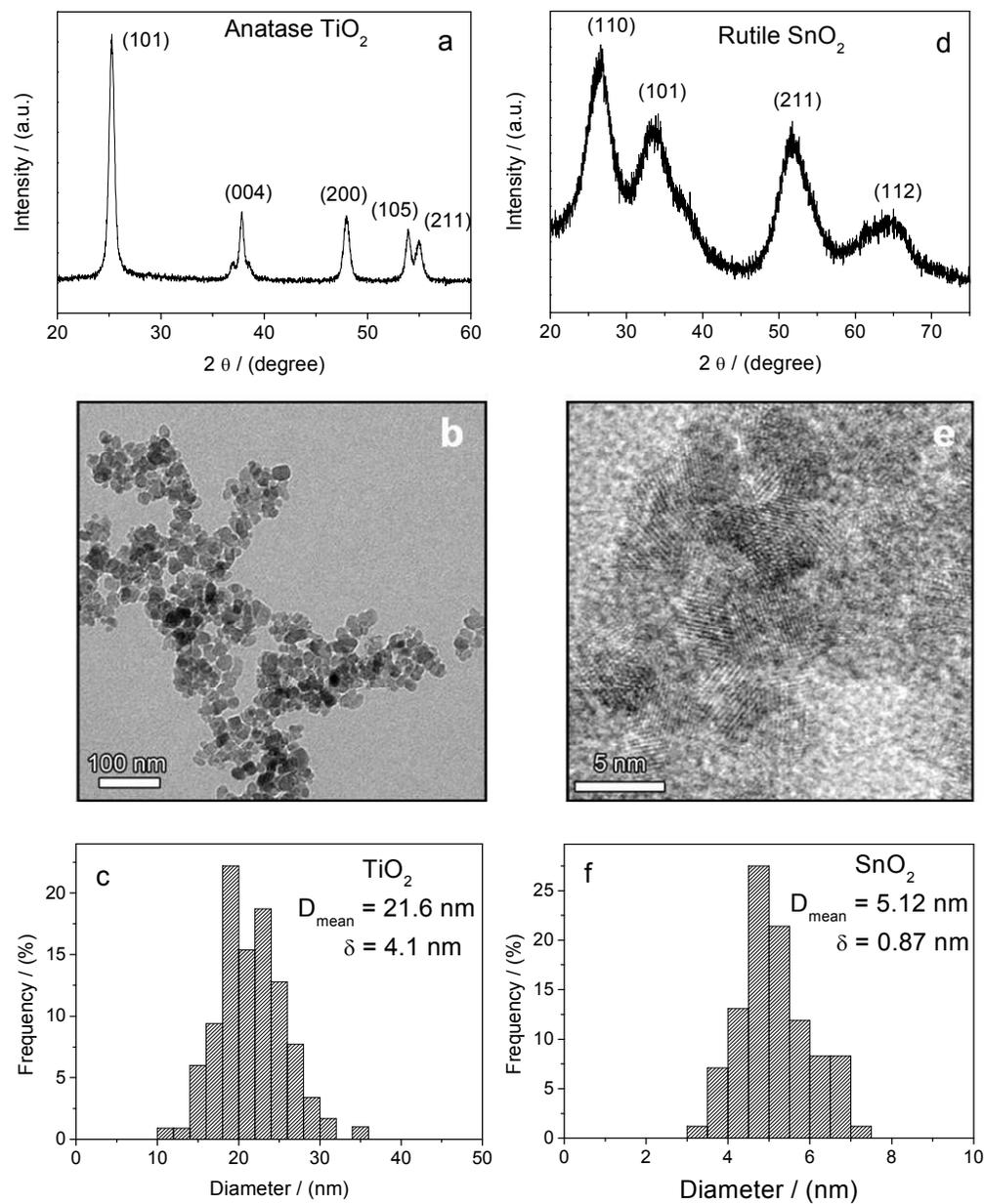
**Figure 1.** Pristine nanoparticle characterization. a) and d) XRD patterns of TiO<sub>2</sub> and SnO<sub>2</sub> nanoparticles; TEM images of b) TiO<sub>2</sub> and e) SnO<sub>2</sub> nanoparticles; c) and f) nanocrystal size distribution obtained from TEM images counting at least 150 particles.
