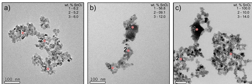
**Figure 2.** TEM images and EDX analyses of selected samples: a) and b) 20 wt. % SnO<sub>2</sub>; c) 50 wt. % SnO<sub>2</sub>. The inset of each panel shows the actual wt. % SnO<sub>2</sub>.
