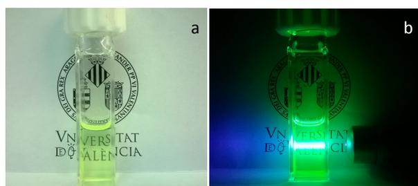
**Fig. 1:** Picture of toluene dispersion of CH<sub>3</sub>NH<sub>3</sub>PbBr<sub>3</sub> nanoparticles under (a) the lab light and (b) UV-laser pointer excitation.
