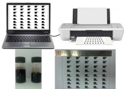
Inkjet printing of conductive Ag-MWCNT patterns and MnO<sub>2</sub>-Ag-MWCNT anodes for supercapacitors.
