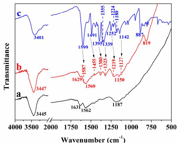
**Fig. 11** FT-IR spectra of PCNS before (a) and after (b) adsorption of MB, and pure MB (c).
