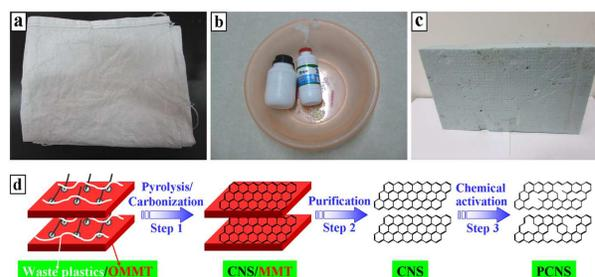
**Fig. 1** Digital images of ubiquitous waste plastics: PP woven bags (a), PE vessels (b) and PS foam sheets (c). Schematic illustration for the process of synthesizing PCNS from the “real-world” mixed waste plastics (d).
