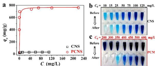
**Fig. 8** (a) Equilibrium adsorption isotherms of MB on the CNS and PCNS (Experimental conditions: MB concentration = 10–125 mg/L for CNS or 200–600 mg/L for PCNS, CNS or PCNS concentration = 0.5 g/L, and adsorption time = 180 min), and the corresponding photos of the MB solutions before and after adsorption by (b) CNS, or (c) PCNS.
