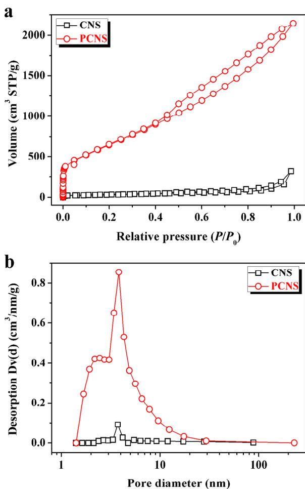
Fig. 4 Nitrogen adsorption/desorption isotherms (a) and pore size distributions (b) of CNS and PCNS.
