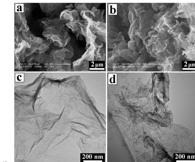
Fig. 2 FE-SEM and TEM images of CNS (a and c) and PCNS (b and d).
