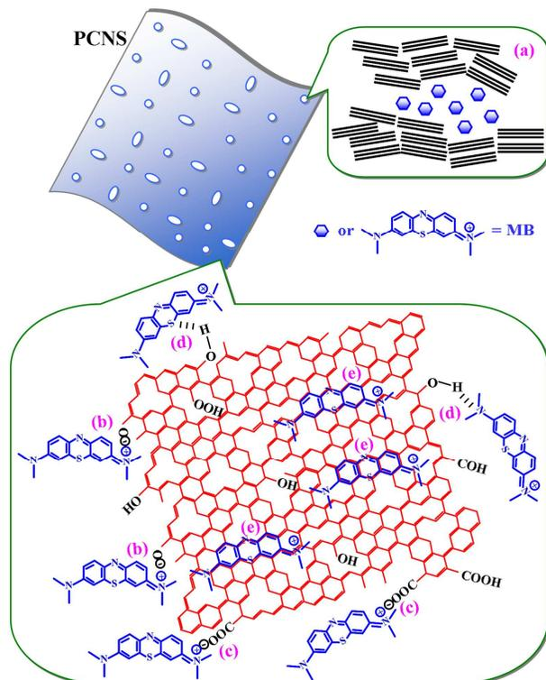
**Fig. 12** Schematic illustration of the interactions between PCNS and MB: (a) pore filling, (b) and (c) electrostatic attraction, (d) hydrogen bonding and (e)  $\pi$ - $\pi$  interactions.
