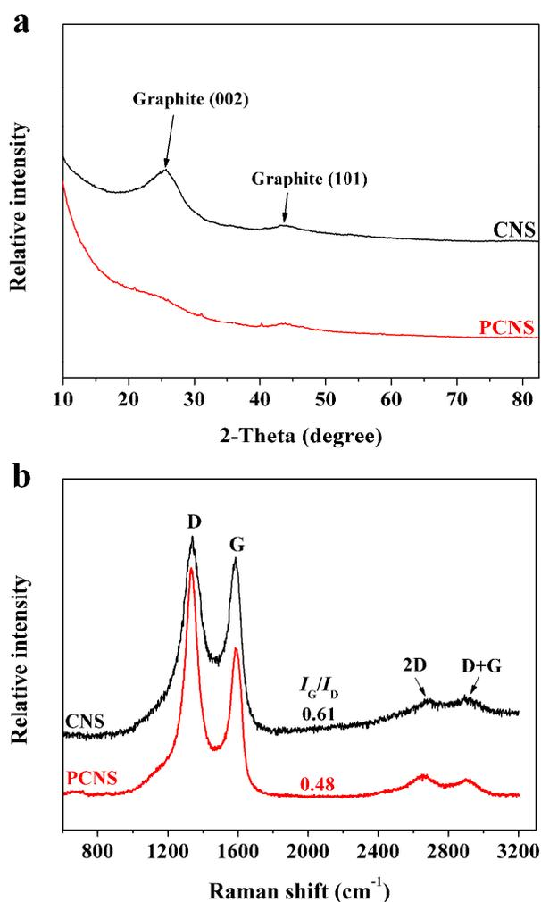
Fig. 5 XRD patterns (a) and Raman spectra (b) of CNS and PCNS.
