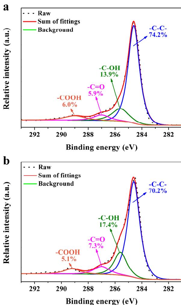
Fig. 6 C 1s high-resolution XPS spectra of CNS (a) and PCNS (b).
