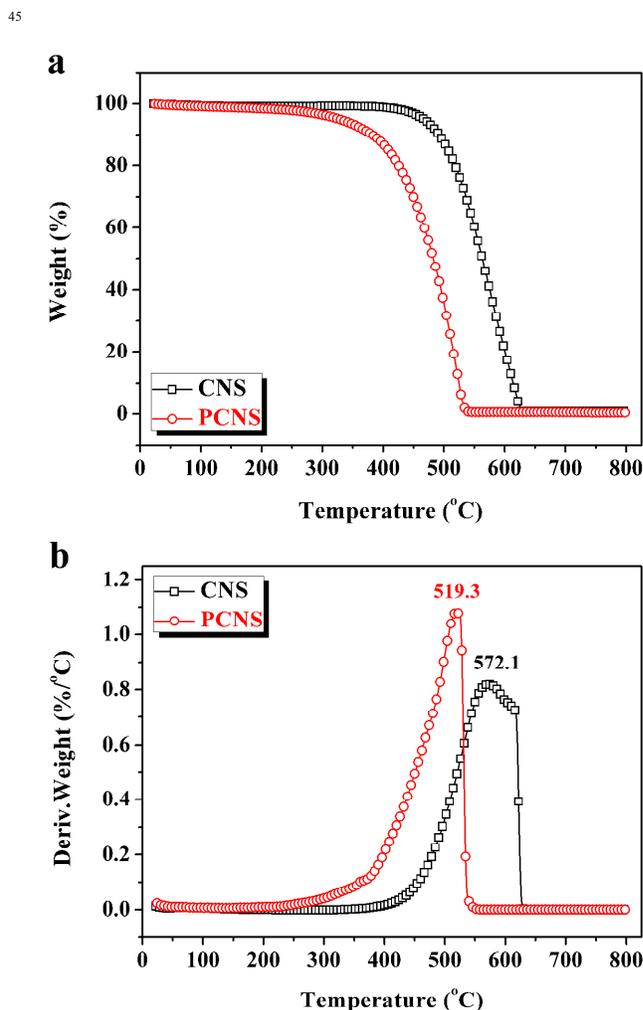
Fig. 7 TGA (a) and DTG (b) curves of CNS and PCNS under air flow at  $10\text{ }^\circ\text{C}/\text{min}$ .
