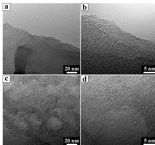
Fig. 3 HR-TEM images of CNS (a and b) and PCNS (c and d).
