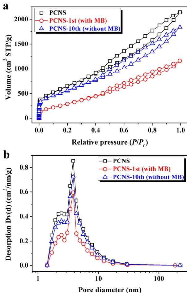
**Fig. 10** Nitrogen adsorption/desorption isotherms (a) and pore size distributions (b) of PCNS before and after MB adsorption (the first cycle), and PCNS after ten cycles.
