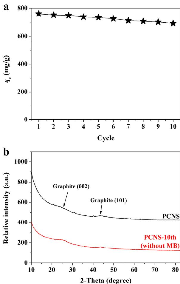
**Fig. 9** (a) The reusability of PCNS for the adsorption of MB (Experimental conditions: MB concentration = 400 mg/L, PCNS concentration = 0.5 g/L, and adsorption time = 180 min), and (b) XRD patterns of PCNS before and after ten cycles.
