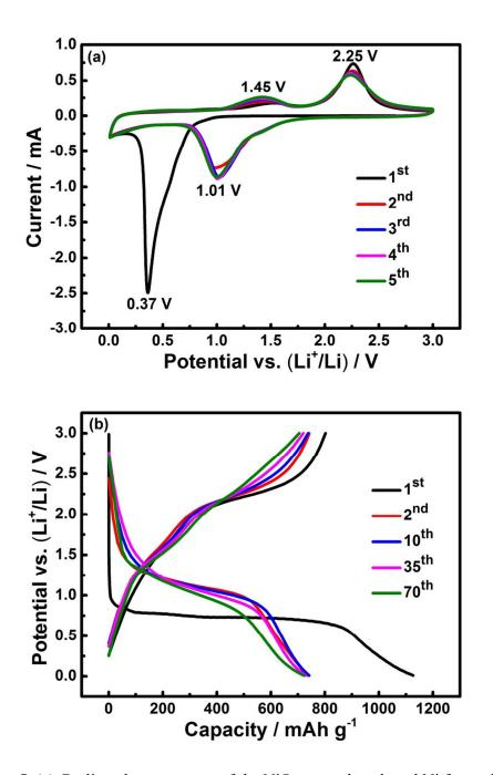
**Figure 5**. (a) Cyclic voltammograms of the NiO nanorod-anchored Ni foam electrode over a potential window of 0.01-3 V (vs.  $\text{Li}^+/\text{Li}$ ) at a scan rate of 0.1 mV s<sup>-1</sup>. (b) Galvanostatic charge-discharge curves of the NiO nanorod-anchored Ni foam at different cycles in a potential range of 0.01-3 V (vs.  $\text{Li}^+/\text{Li}$ ) at a current density of 1 A  $g^{-1}$ .
