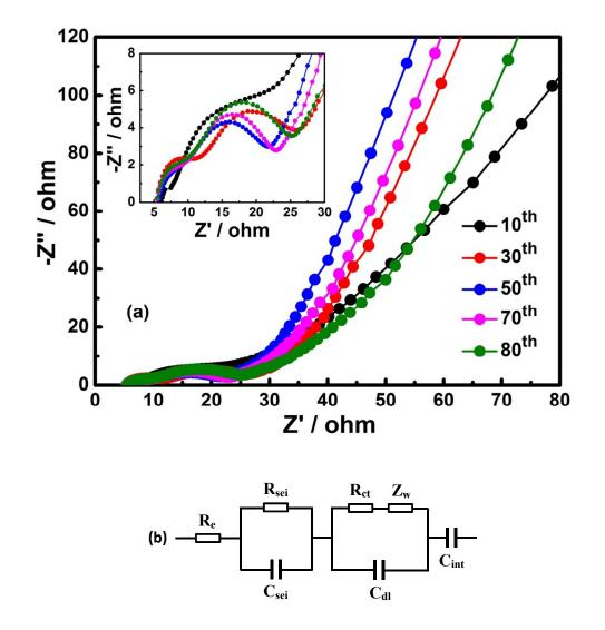
**Figure 8.** (a) Nyquist plots of the NiO nanorod-anchored Ni foam electrode after different cycles at a current density of 1 A  $g^{-1}$  in the charged state (3 V vs. Li<sup>+</sup>/Li) over the frequency range of 0.01 Hz-100 kHz. Inset of (a) shows the enlarged parts at high frequency region. (b) Equivalent electrical circuit corresponding to the Nyquist plots.
