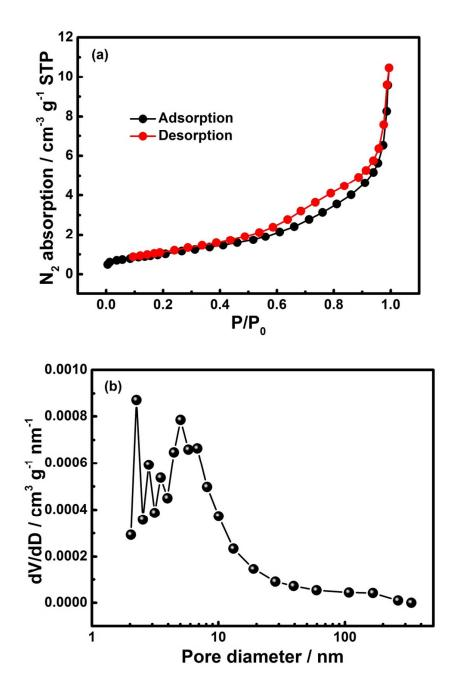
**Figure 4**. (a) N<sub>2</sub> adsorption-desorption isotherms and (b) pore size distribution of the NiO nanorod-anchored Ni foam electrode (based on the total mass of the electrodes).
