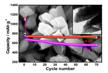
3D binder-free NiO nanorod-anchored Ni foam electrodes synthesized by in-situ anodization and annealing exhibit superior cyclability and high rate performance.
