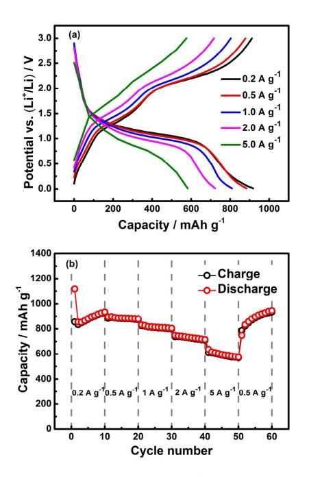
**Figure 7.** (a) Representative charge-discharge profiles of the NiO nanorod-anchored Ni foam electrode at varied current densities. (b) Rate performance of the NiO nanorod-anchored Ni foam electrode at varied current densities.
