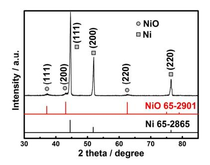
Figure 1. XRD pattern of the NiO nanorod-anchored Ni foam electrode.
