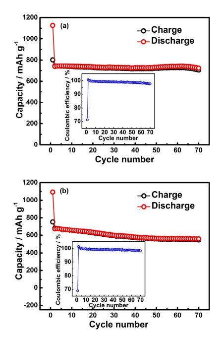
**Figure 6**. Cycling performance of the NiO nanorod-anchored Ni foam electrode at a current density of (a)  $1 \text{ A g}^{-1}$  and (b)  $2 \text{ A g}^{-1}$ . Insets of (a, b) show the corresponding coulombic efficiency.
