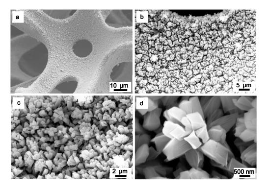
Figure 2. SEM images of the NiO nanorod-anchored Ni foam electrode.
