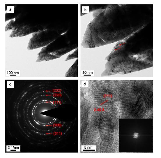
**Figure 3.** (a, b) TEM images, (c) SAED pattern and (d) HRTEM image of the NiO nanorod-anchored Ni foam electrode. Inset of (d) shows the FFT pattern corresponding to the HRTEM image.
