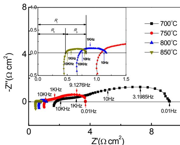
**Figure 9** EIS of MT-SOFC at different temperatures under open circuit condition.
