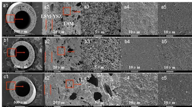
**Figure 1** Microstructure of LSM-YSZ/LSM dual-layer hollow fiber membranes sintered at different temperatures. a-sintering at 1300°C; b- sintering at 1350°C; c- sintering at 1400°C; (1) cross-section; (2)Interface of LSM-YSZ/LSM; (3) Microstructure of LSM layer; (4) inner surface; and (5) outer surface.
