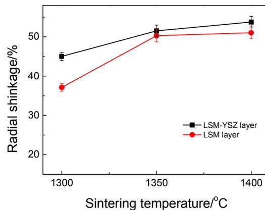
**Figure 2** Radial shrinkage of LSM & LSM-YSZ layer as a function of sintering temperature.
