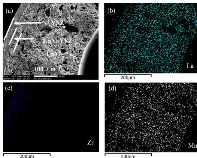
**Figure 5** Microstructure and X-ray energy dispersive spectrometry (EDX) analysis of YSZ/CFL/LSM tri-layer membrane sintered at 1350 °C, (a) cross section, (b) La mapping; (c) Zr mapping, (d) Mn mapping.
