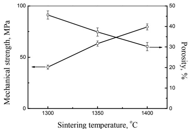
**Figure 3** Porosity and mechanical strength of the dual-layer LSM-YSZ/LSM hollow fiber at different sintering temperature.
