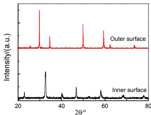
**Figure 6** XRD of inner surface and outer surface of the YSZ/CFL/LSM tri-layer membrane.
