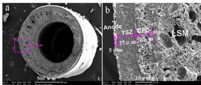
**Figure 7** Microstructure of dual-layer cathode-supported MT-SOFC. (a) cross-section; (b) anode/electrolyte/CFL/LSM interface.
