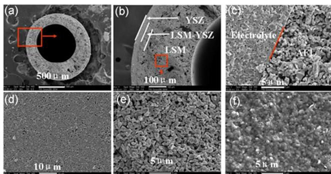
**Figure 4** Microstructure of the YSZ/CFL/LSM tri-layer hollow fibers sintered at 1350°C. (a) over-view; (b) cross-section; (c) interface of YSZ/CFL; (d) inner surface; (e) LSM layer; (f) outer surface.
