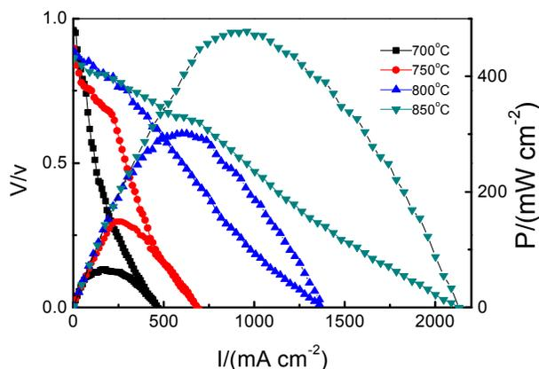
**Figure 8** Output of MT-SOFC based on the LSM-YSZ/LSM dual-layer hollow fibers ( $\text{H}_2$  feed flow rate =  $40 \text{ mL min}^{-1}$ ; air feed flow rate =  $90 \text{ mL min}^{-1}$ ).
