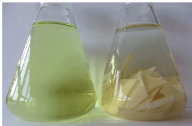
Figure 2. Chromate solutions ( 50 \text{ mg L}^{-1} , pH 5) before (left) and after addition (right) of PVAm@PET. The discoloration of the solution is easily recognizable.
