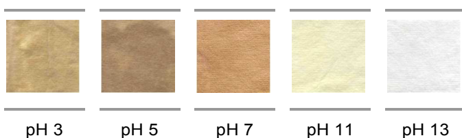
Figure 3. 4 % PVAm@PET fabrics after adsorption of chromate at different pH values.
