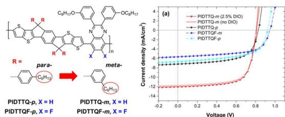
Two pairs of novel indacenodithieno[3,2-*b*]thiophene (IDTT) and quinoxaline based copolymers with *meta*- or *para*-hexyl-phenyl side chains on the IDTT unit are synthesized for enhanced photovoltaic performance.
