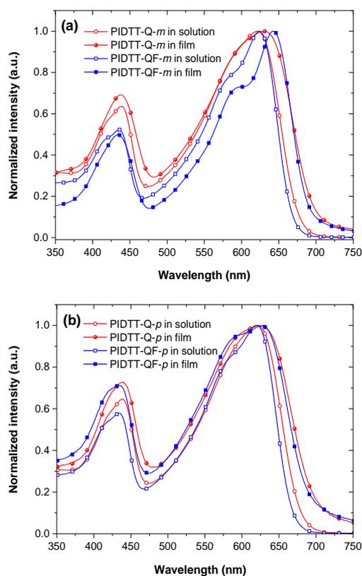
**Fig. 1** Normalized UV-Vis absorption spectra of the polymers (a) *meta*-substituted polymer PIDTT-Q-
