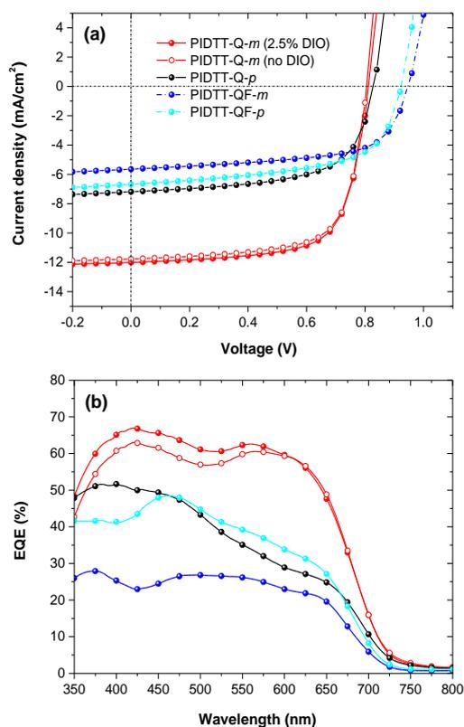
**Fig. 3** (a) Current density-voltage characteristics of IDTT copolymer:PC<sub>71</sub>BM solar cells; (b) External quantum efficiency (EQE) spectra measured under illumination of monochromatic light.
