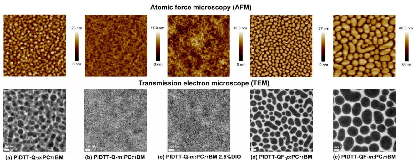
**Fig. 4** AFM and TEM topography images of optimized IDTT copolymer:PC<sub>71</sub>BM blended layers.
