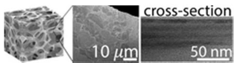
Single bilayer polymer/clay nanobrick wall self-assembled thin films, deposited as a continuous coating on open-celled polyurethane foam, cut peak heat release rate in half with only 3.2 wt% addition.
