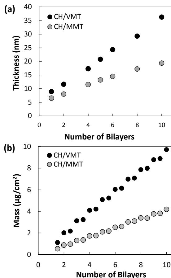
**Fig. 1** a) Film thickness and b) mass as a function of bilayers deposited for polymer/clay assemblies. Ellipsometry was used to measure thickness, while QCM measured mass.
