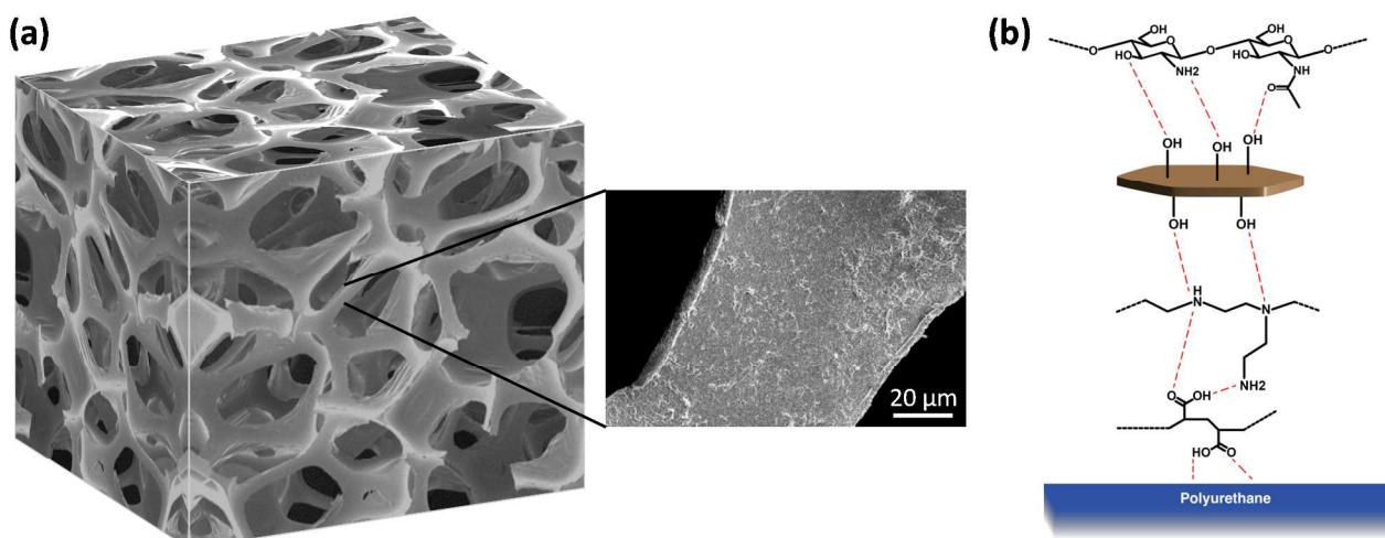
**Fig. 5** Schematic of the coated foam (inset: SEM image of 4 BL MMT-based nanobrick wall on polyurethane). b) Chemical structures of the nanobrick wall components after deposition (PAA surface treatment, PEI primer, clay, and chitosan).
