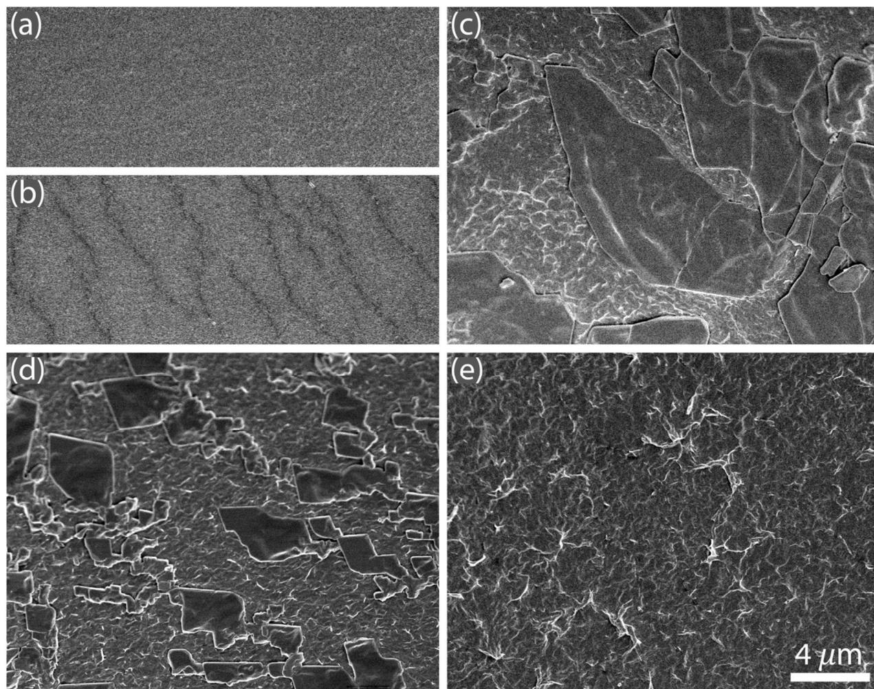
**Fig. 2** SEM images of a) control foam, foam coated with b) a single layer of PEI, c) a single PEI/VMT bilayer, d) a single PEI/MMT bilayer, and e) a 4 BL MMT-based coating.
