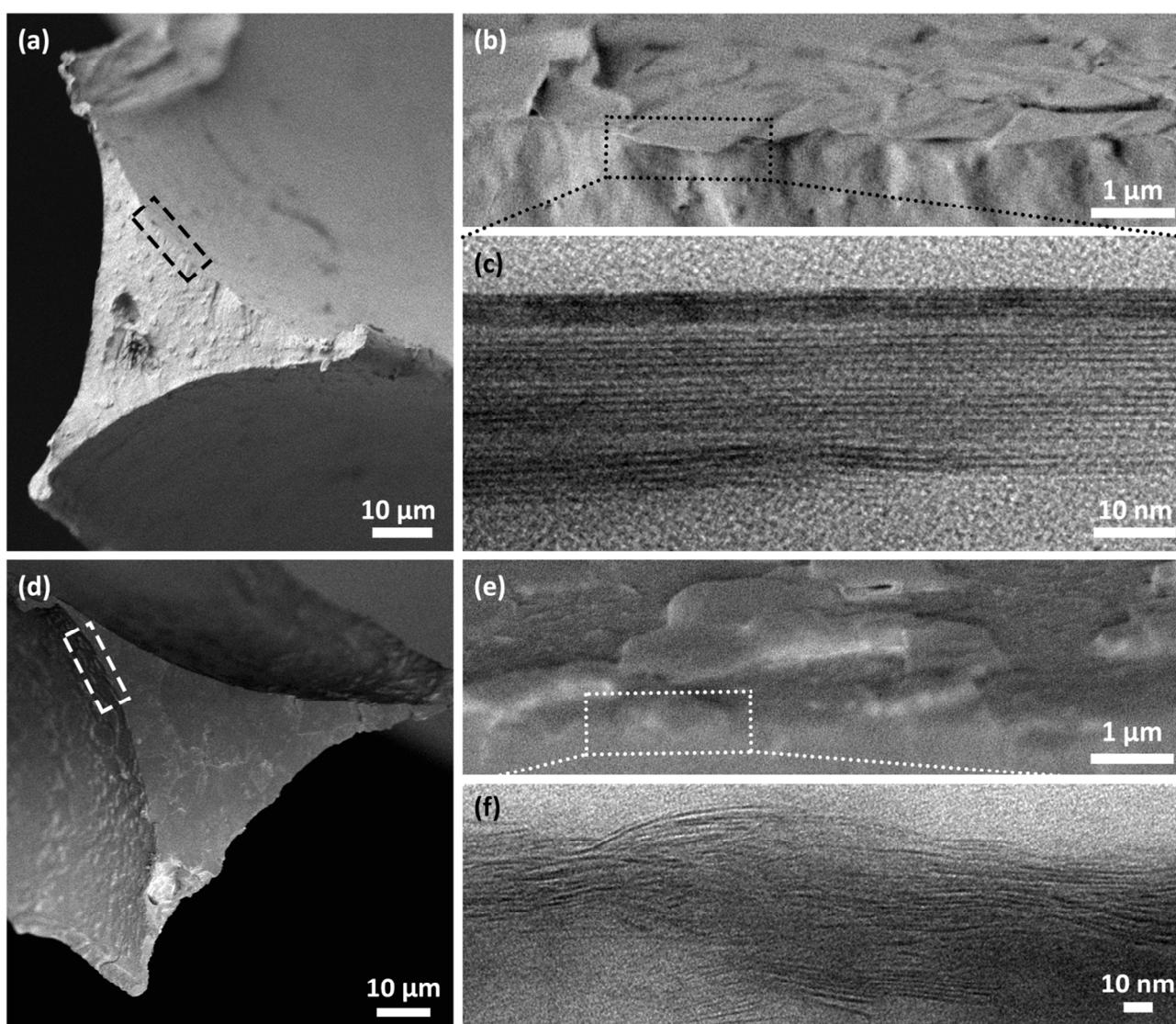
**Fig. 3** SEM images of freeze-fractured polyurethane foam coated with 1 BL of a-b) PEI/VMT and d-e) PEI/MMT. TEM micrographs of polyurethane foam coated with 1 BL of c) PEI/VMT and f) PEI/MMT.
