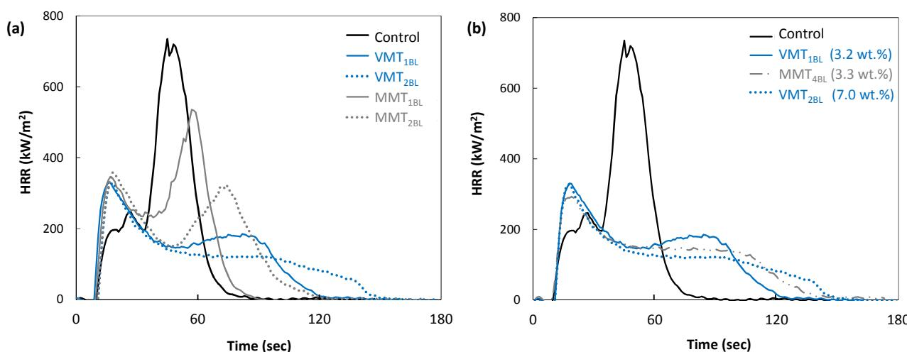
**Fig. 4** Heat release rate as a function of time for control foam and foam coated with nanobrick wall thin films with varying a) number of layers deposited and b) coating weight addition.
