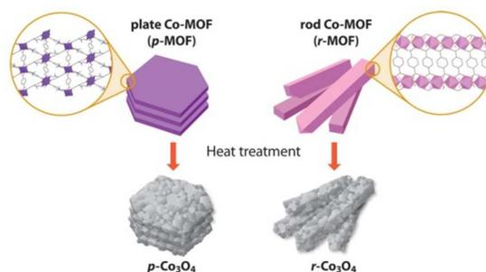
Pseudomorphic conversion of MOFs resulted in the controlled preparation of  $\text{Co}_3\text{O}_4$  nanoparticles with different microstructures, which showed different electrochemical properties.
