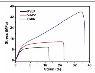
Fig. 2 Stress-strain curves of the as-prepared electrospun PVdF, V/M/V and PMIA nanofibrous membranes.
