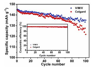
**Fig. 8** Cycle performance of the cells assembled with the resultant composite membranes and Celgard membrane at 0.2C rate. Inset shows the coulombic efficiency as a function of the number of cycles.
