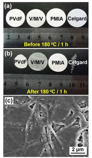
Fig. 4 Photographs of electrospun nanofibrous membranes and Celgard membrane (a) before and (b) after exposure to 180  $^\circ C$  for 1 h, (c) FE-SEM image of the composite membranes after being exposed to 180  $^\circ C$  for 1 h.
