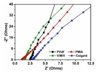
Fig. 6 AC impedance spectra of liquid electrolyte-soaked electrospun PVdF, V/M/V, PMIA nanofibrous membranes and Celgard membrane.
