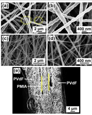
Fig. 1 FE-SEM images of (a and b) PVdF, (c and d) PMIA nanofibrous membranes. (e) FE-SEM image of the cross-section view of V/M/V composite membranes.
