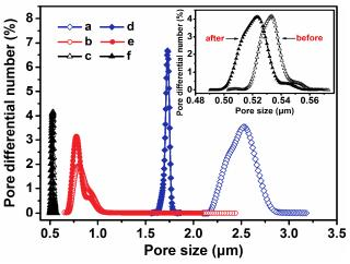
Fig. 5 Pore size distributions of electrospun PVdF (a and d), V/M/V (b and e), and PMIA (c and f) membranes before (a, b and c) and after (d, e and f) being exposed to 180 °C for 1 h. Inset shows the region (0.480-0.578  $\mu$ m).
