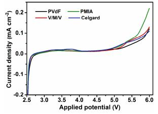
Fig. 7 Electrochemical stability windows of the cells with as-prepared PVdF, V/M/V, PMIA nanofibrous membranes and Celgard membrane.
