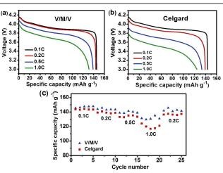
**Fig. 9** Discharge curves of the cells assembled with (a) V/M/V composite membranes and (b) Celgard membrane as separators at different C-rate, (c) Comparison of the rate capabilities.
