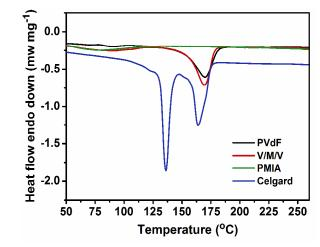
Fig. 3 DSC curves of Celgard membrane and the resultant electrospun PVdF, V/M/V, and PMIA nanofibrous membranes.
