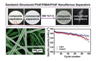
Novel, sandwich structured PVdF/PMIA/PVdF nanofibrous battery separators with robust mechanical strength and thermal stability are fabricated via a sequential electrospinnning technique.
