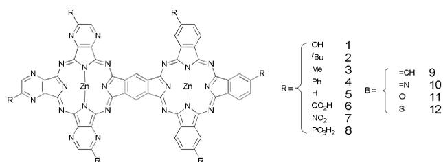
Fig 13. Molecular structures of fused ZnPc-based sensitizers.
