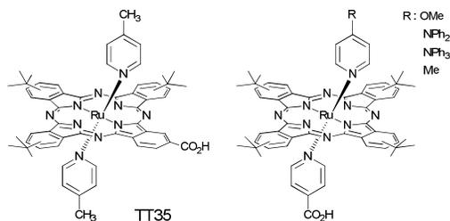
Fig 8. Molecular structure of RuPc based sensitizers.
