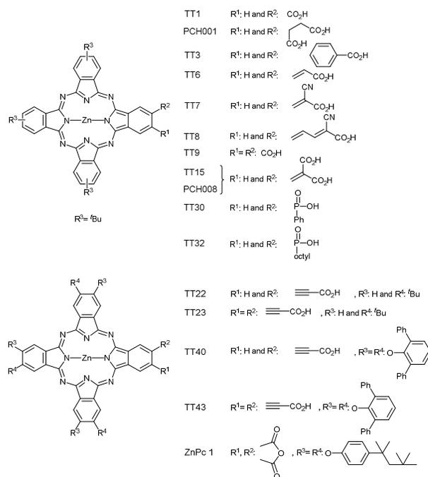
Fig. 6. Molecular structures of the ZnPc-based sensitizers.
