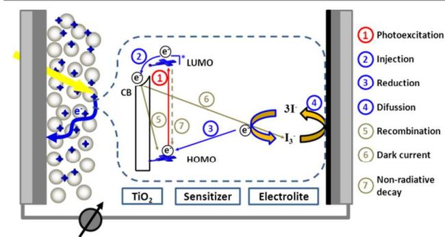
Fig. 1 Schematic representation of the composition and the operating principle of a DSSC.
