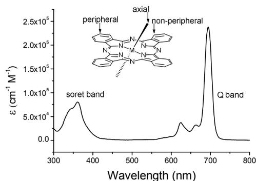
Fig. 3. Typical structure of a phthalocyanine showing the non-peripheral, peripheral and axial positions to be functionalized for phthalocyanine-sensitized solar cells, together with a typical UV-vis spectrum of a metallophthalocyanine.
