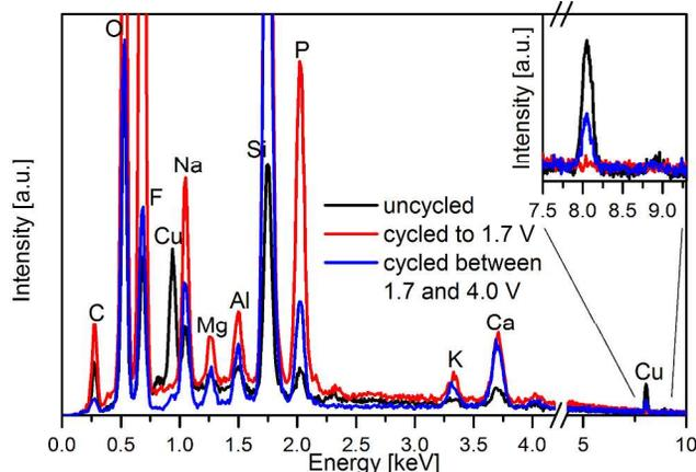
Figure 9: EDX spectra of lithium counter electrodes to working electrodes of  $\text{Cu}_{0.5}\text{TiOPO}_4$  after cycling to 1.7 V, cycling for 10
