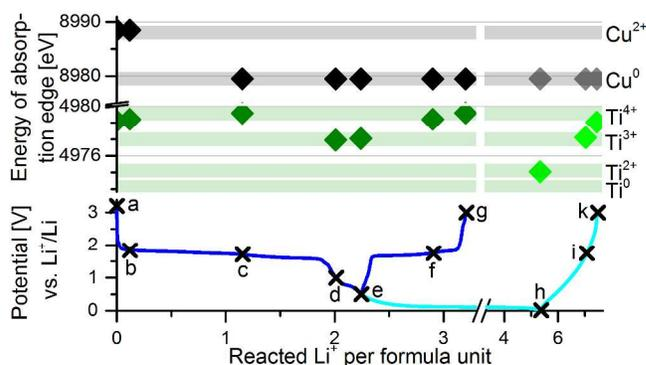
Figure 6: Change of the energy of the copper- and titanium absorption edge at half of the edge step of ex situ samples of  $\text{Cu}_{0.5}\text{TiOPO}_4$ . The position of the absorption edge of the measured reference materials is shown as well. At the bottom, the corresponding galvanostatic curve is plotted.
