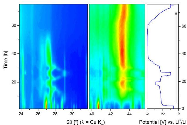
Figure 2: Contour plot of an in situ XRD measurement at a specific current of 16.9 A/kg (blue: low intensity; red: high intensity). On the right hand side, the corresponding galvanostatic curve is shown.
