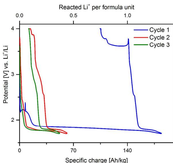
Figure 8: Galvanostatic curve of  $\text{Cu}_{0.5}\text{TiOPO}_4$  cycled for 3 cycles between 1.7 V and 4.0 V with a specific current of 14.06 A/kg.
