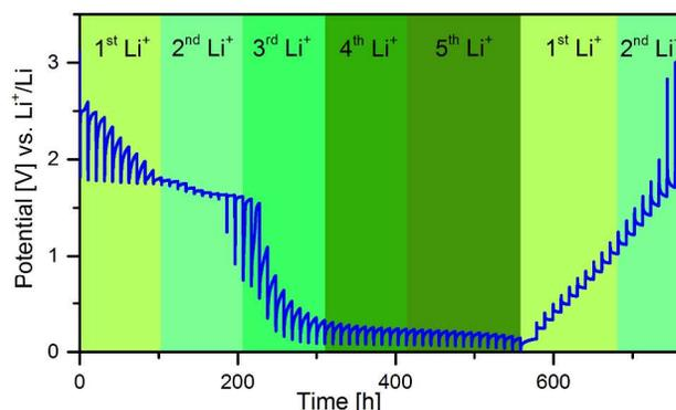
Figure 1: GITT-measurement during the first cycle.
