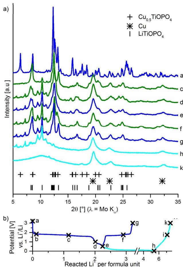
Figure 3: a) Ex situ XRD measurements of  $\text{Cu}_{0.5}\text{TiOPO}_4$  cycled to key points in the first cycle. b) shows the corresponding galvanostatic curve.
