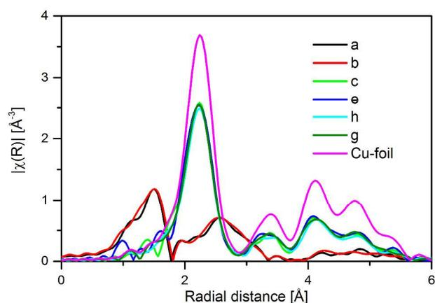
Figure 4: Fourier transform of the recorded EXAFS-spectra of cycled samples of  $\text{Cu}_{0.5}\text{TiOPO}_4$  (for labeling see Figure 6).
