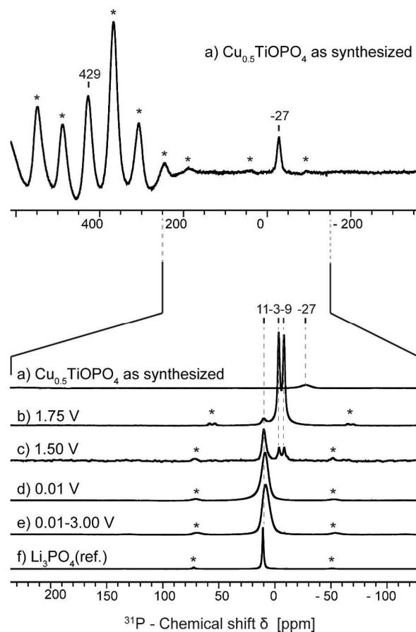
Figure 7:  $^{31}\text{P}$  MAS NMR spectra of ex situ samples of  $\text{Cu}_{0.5}\text{TiOPO}_4$  and pure  $\text{Li}_3\text{PO}_4$ . The top spectrum is an addition of two spectra acquired at two different transmitter positions (0 ppm and 250 ppm) to cover a larger window width. For all the spectra the number of scans was 512K and the recycling delay was set to 1 s.
