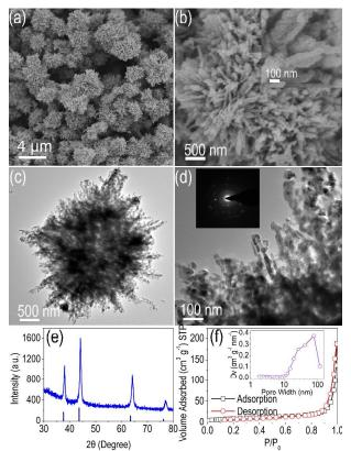
Fig.3 Morphology and structure characterization of urchin-like Co(OH)<sub>2</sub>:
