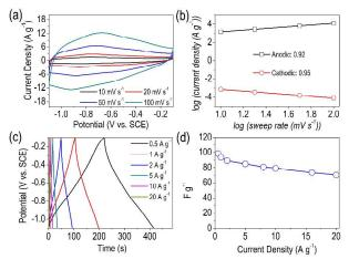
Fig.4 Electrochemical characteristics of urchin-like VN in 2M KOH electrolyte under a three-electrode system: (a) CV curves at the scan rates,
