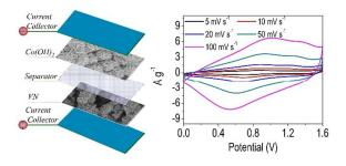
**Text:** A new hybrid supercapacitor with excellent electrochemical performance is fabricated by using the flower-like  $Co(OH)_2$  and urchin-like VN.
