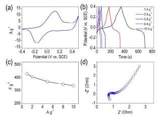
Fig.2 Electrochemical characteristics of flower-like Co(OH)<sub>2</sub> in 2M KOH electrolyte under a three-electrode system: (a) typical CV curve at the scan rate of 10 mV s<sup>-1</sup>, (b) galvanostatic charge/discharge curves at different current densities, (c) the specific capacitance as a function of the discharge current density, and (d) Nyquist plot showing the imaginary part versus the real part of impedance
