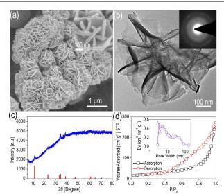
Fig.1 Morphology and structure characterization of flower-like Co(OH)<sub>2</sub>:
