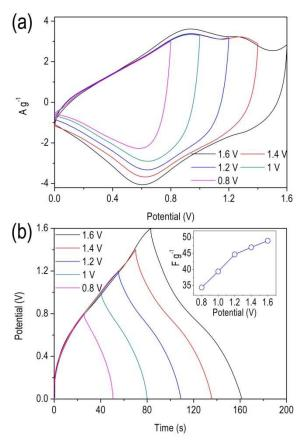
Fig.6 (a) CV (scan rate of 50 mV s<sup>-1</sup>) and (b) galvanostatic charge/discharge curves (current density of 1 A g<sup>-1</sup>) of an optimized Co(OH)<sub>2</sub>//VN hybrid supercapacitor (VN/Co(OH)<sub>2</sub> mass ratio: 3)
