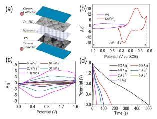
Fig.5 (a) Schematic of the assembled structure of hybrid supercapacitor based on the flower-like Co(OH)<sub>2</sub> as the positive electrode and urchin-like VN as the negative electrode. (b) Cyclic voltammetry profiles for
