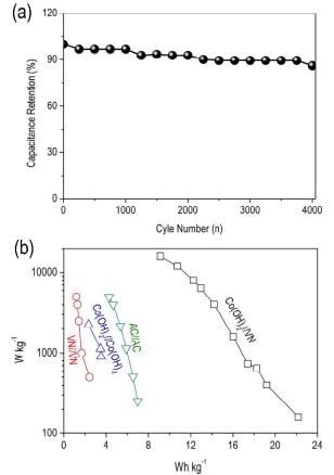
Fig.8Plot of cycle stability of Co(OH)<sub>2</sub>//VN hybrid supercapacitor with the VN/Co(OH)<sub>2</sub> mass ratio of 3 at the current load of 1 A g<sup>-1</sup> (b) Ragone plot (power density vs. energy density) of hybrid supercapacitor made of Co(OH)<sub>2</sub> and VN. Comparison of supercapacitor composed of VN//VN, Co(OH)<sub>2</sub>//Co(OH)<sub>2</sub>, and commercial AC//AC (AC from *ShiheziTianfu Tech Co., Ltd,China*).
