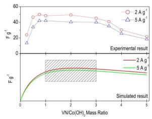
Fig.7 Plots of specific capacitance with VN/Co(OH)<sub>2</sub> mass ratio of hybrid supercapacitor from experimental results and simulated results from Wilson' mathematical model. The shadow area shows the maximum specific capacitance area of hybrid supercapacitor
