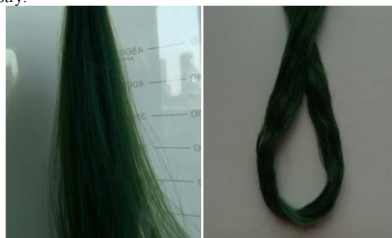
Fig. 1 Photographs of the wet PANI/ cellulose multifilament fibers in distilled water (left) and the dried PANI/cellulose multifilament fibers (right) spun from PANI/cellulose solution.
