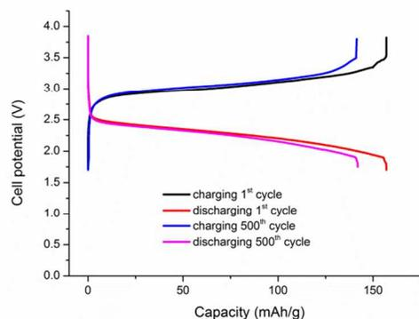
Figure 2: Charge/discharging curves (capacity vs. potential) of the Li-organic battery of the 1<sup>st</sup> and the 500<sup>th</sup> cycle (solid line). The anode is lithium metal, the cathode is a composite with polyTCAQ **5** as active material.
