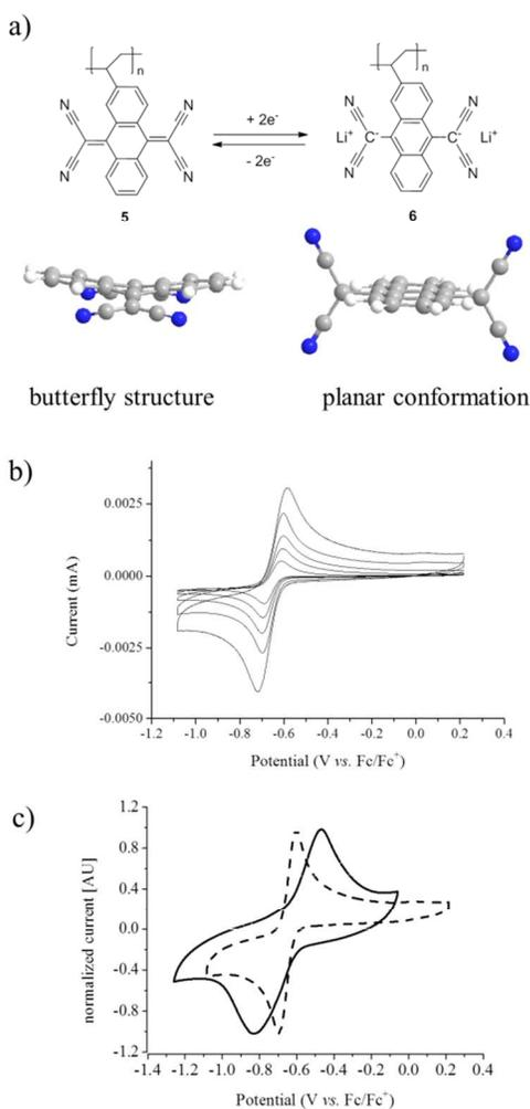
Figure 1: a) Schematic representation of the redox couple of polyTCAQ (**5**). b) Cyclic voltammogram of monomer **4** in propylene carbonate, 0.1 M lithium perchlorate at different scan rates (10, 25, 50, 100 and 250 mV/s, respectively). c) Normalized cyclic voltammograms of the monomer **4** in solution (dashed line) and a polymer-composite electrode (solid line) (10/80/10 wt% 5/VGCF/PVdF) in propylene carbonate, 0.1 M lithium perchlorate.
