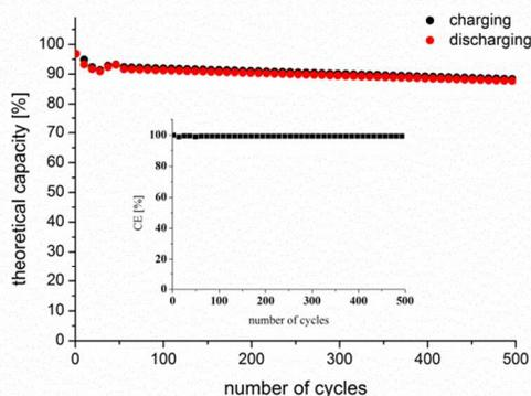
Figure 3: Extended charge/discharge cycling of **5** in propylene carbonate, 0.1 M lithium perchlorate (500 cycles, 1 C). Coulombic efficiency (CE%) of 500 charge/discharge cycles (black squares).
