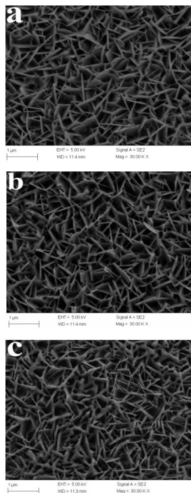
Fig. 3 SEM images of (a) 2.5% W doped \text{BiVO}_4 film, (b) 5% Mo doped \text{BiVO}_4 film and (c) 2%W, 6% Mo co-doped \text{BiVO}_4 film.
