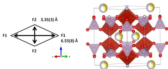
**Figure 12.** Crystal structure of the cathode at the 4.3 V charged state during the potentiostatic step. PO<sub>4</sub> are shown in purple and VO<sub>4</sub>F<sub>2</sub> in red.
