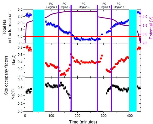
**Figure 13.** Evolution of Na(1) (in black), Na(2) (in red) and total sodium content (in blue) as a function of time and electrochemical processes in the pre-cycled cell containing the Na<sub>3</sub>V<sub>2</sub>O<sub>2x</sub>(PO<sub>4</sub>)<sub>2</sub>F<sub>3-2x</sub> electrode.
