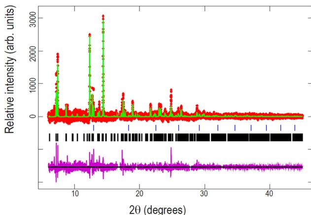
**Figure 7.** Rietveld refinement of the  $\text{Na}_3\text{V}_2\text{O}_{2x}(\text{PO}_4)_2\text{F}_{3-2x}$  model to the synchrotron XRD data of the pre-cycled cell before *in-situ* cycling. Data are shown as crosses, the calculated Rietveld model as a line through the data, and the difference between the data and the model as the line below the data. The vertical reflection markers are for  $\text{Na}_3\text{V}_2\text{O}_{2x}(\text{PO}_4)_2\text{F}_{3-2x}$ .
