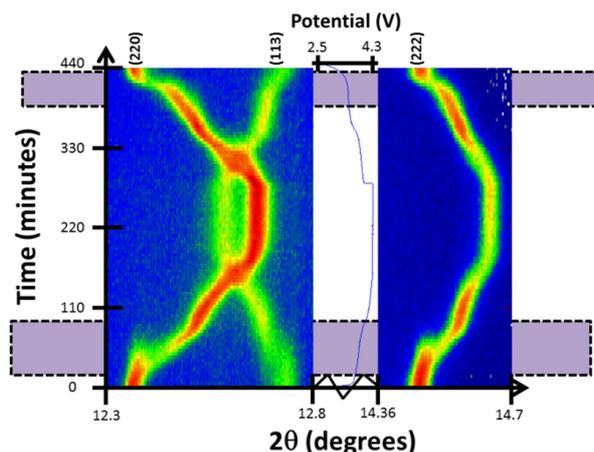
**Figure 8.** Two-dimensional plots of (220), (113) and (222) reflections versus time and voltage. Purple shaded areas mark two-phase regions where there are two sets of reflections.
