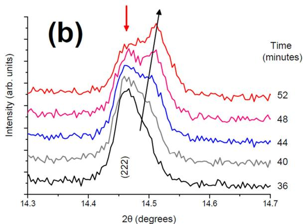
**Figure 9.** Diffraction patterns from 36 to 52 minutes in the  $2\theta$  ranges of a) (220) and b) (222) reflection.
