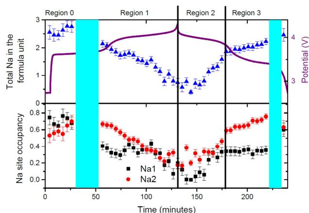
**Figure 5.** Evolution of Na(1) (in black), Na(2) (in red) and total sodium content (in blue) in the fresh  $\text{Na}_3\text{V}_2\text{O}_{2x}(\text{PO}_4)_2\text{F}_{3-2x}$  electrode. Regions are defined at the top and correspond to solid solution type reactions. Turquoise shaded areas represent two-phase transition stages.
