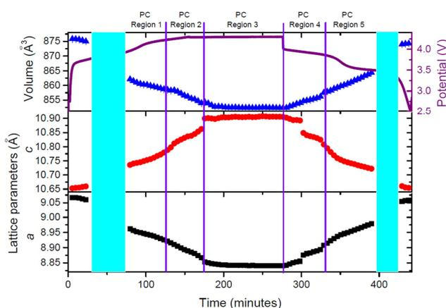
**Figure 11.** Evolution of the lattice parameters and unit-cell volume of the cathode of the pre-cycled cell as a function of time, with the potential profile included. Regions are defined at the top and correspond to solid solution type reactions. Blue shaded areas represent two-phase transitions.
