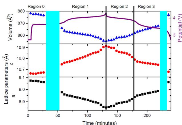
**Figure 4.** Evolution of lattice parameters and unit cell volume of the fresh cell cathode as a function of time, with the potential profile included.
