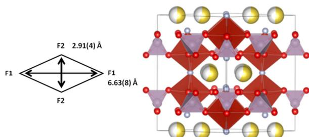
**Figure 14.** Crystal structure of the cathode at the end of the upper voltage solid solution.  $\text{PO}_4$  are shown in purple and  $\text{VO}_4\text{F}_2$  in red. Oxygen is red, fluorine is light blue and sodium is yellow with the shading indicating occupancy. Channel size in the  $xy$  plane is indicated in the scheme.
