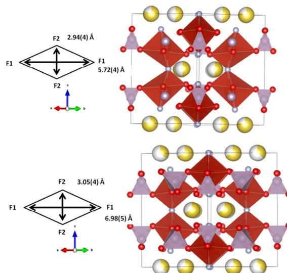
**Figure 10.** Refined structures of pre-SS1 (top) and pre-SS2 (bottom). PO<sub>4</sub> are shown in purple and VO<sub>4</sub>F<sub>2</sub> in red. Oxygen is red, fluorine is light blue and sodium is yellow with the shading indicating occupancy. Channel size in the  $xy$  plane is indicated in the schemes.
