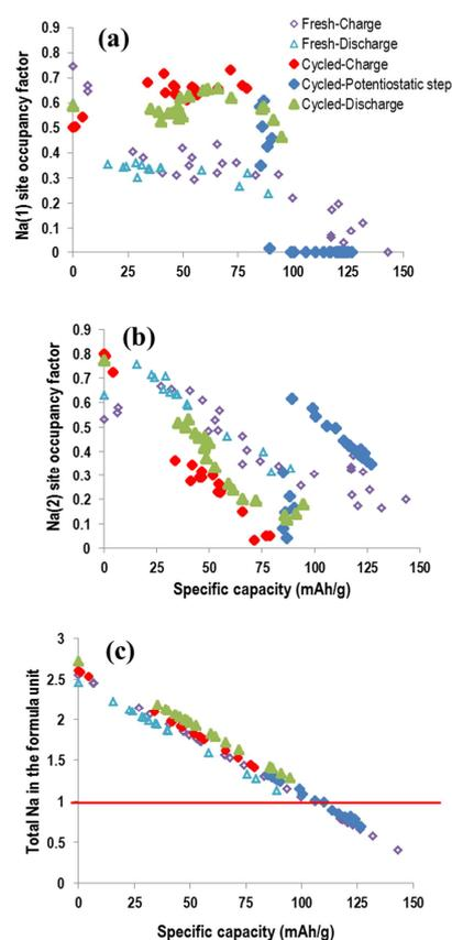
**Figure 15.** Sodium occupancies (a, b) and total content (c) *vs.* specific capacity for the fresh and pre-cycled cell.
