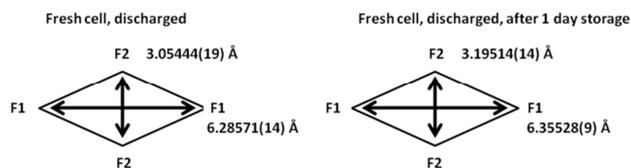
**Figure 6.** Channel size in the *xy* plane for the discharged fresh cell cathode and the same material stored in the coin cell for 1 day.
