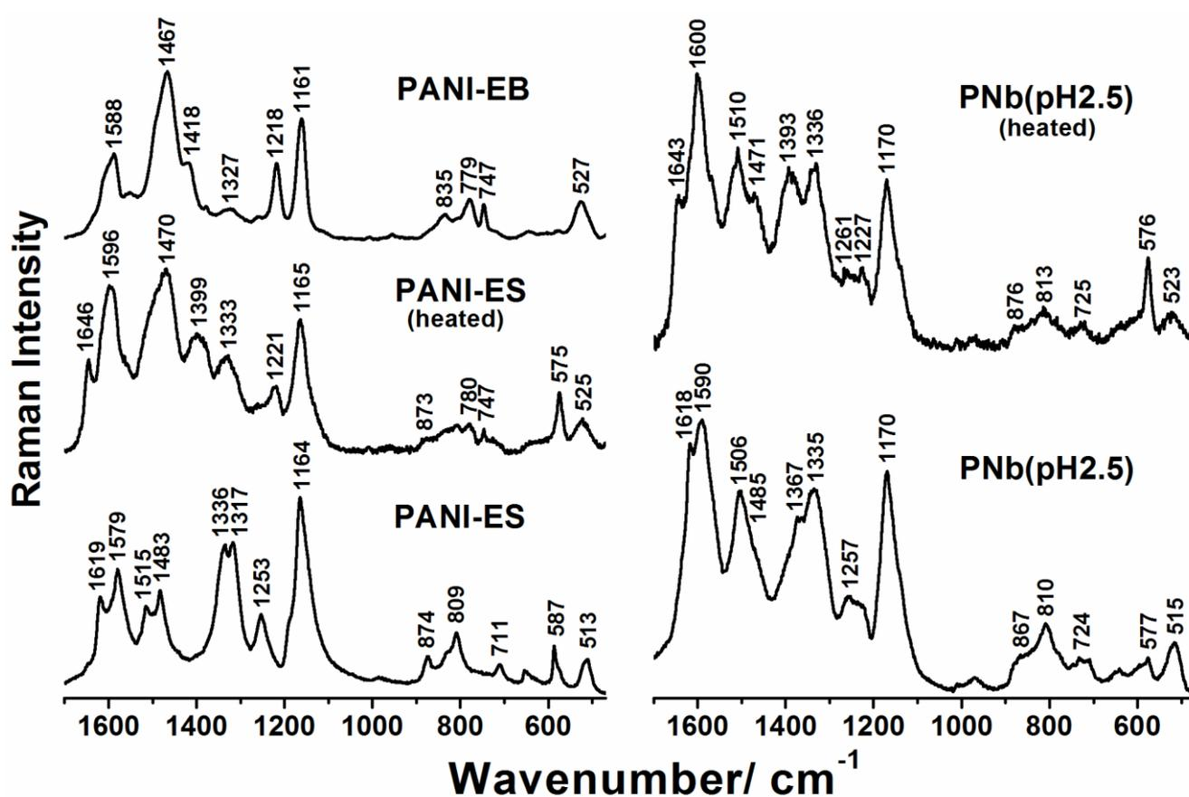
Figure 8. Resonance Raman spectra ( $\lambda_0 = 632.8 \text{ nm}$ ) of PANI-ES and hybrid material PNb(pH2.5) before and after heating treatments (150  $^{\circ}\text{C}$  during 90 min). For comparison purposes, the Raman spectrum of PANI-EB is also presented. See the RR spectrum of hybrid material PNb(pH0.1) in Supporting Information (figure S3).
