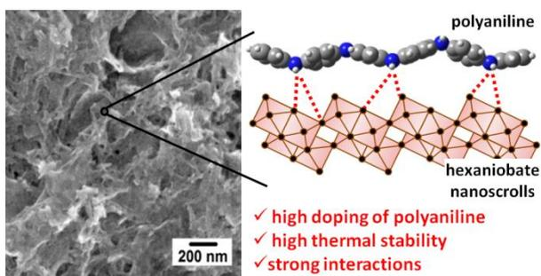
New hybrid materials of polyaniline and hexaniobate nanoscrolls were prepared by mixture of the dispersions. These materials show high doping of polyaniline and high thermal stability.
