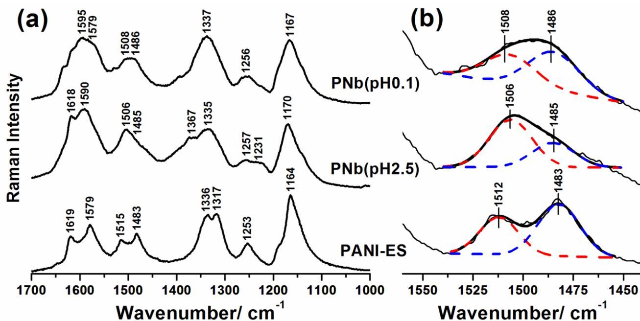
Figure 5. (a) Resonance Raman spectra ( $\lambda_0 = 632.8$  nm) of PANI-ES and the hybrid materials PNB(pH2.5) and PNB(pH0.1) at 1700-1000  $\text{cm}^{-1}$  range. (b) Peak fitting of Raman bands at 1550-1450  $\text{cm}^{-1}$  range (dashed lines).
