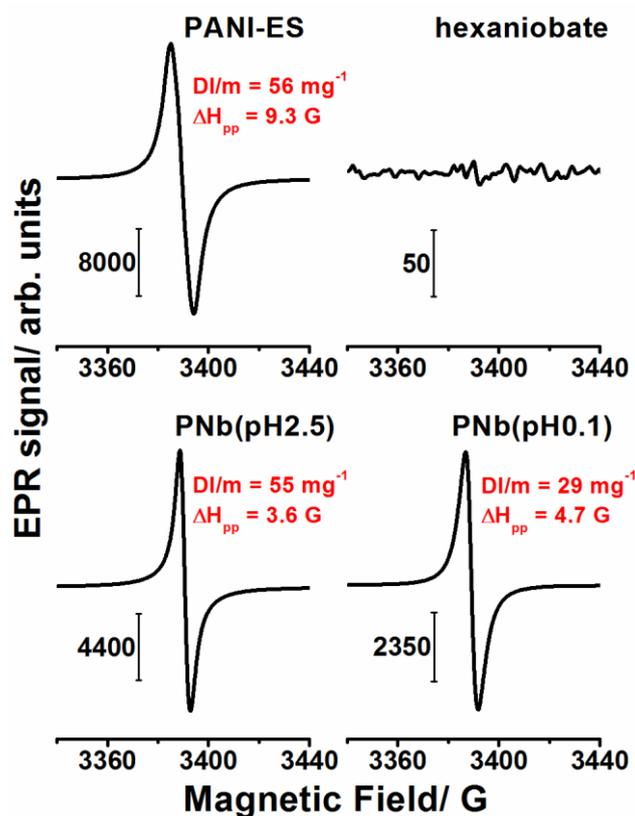
Figure 6. EPR spectra of PANI-ES, hexaniobate and hybrid materials PNb(pH2.5) and PNb(pH0.1).  $DI/m$  and  $\Delta H_{pp}$  are the values of the EPR signal (integral areas of the EPR signals normalized by the weight of polymer) and the EPR linewidth, respectively. For details of sample weights and polymer contents, see Supporting Information (table S1).
