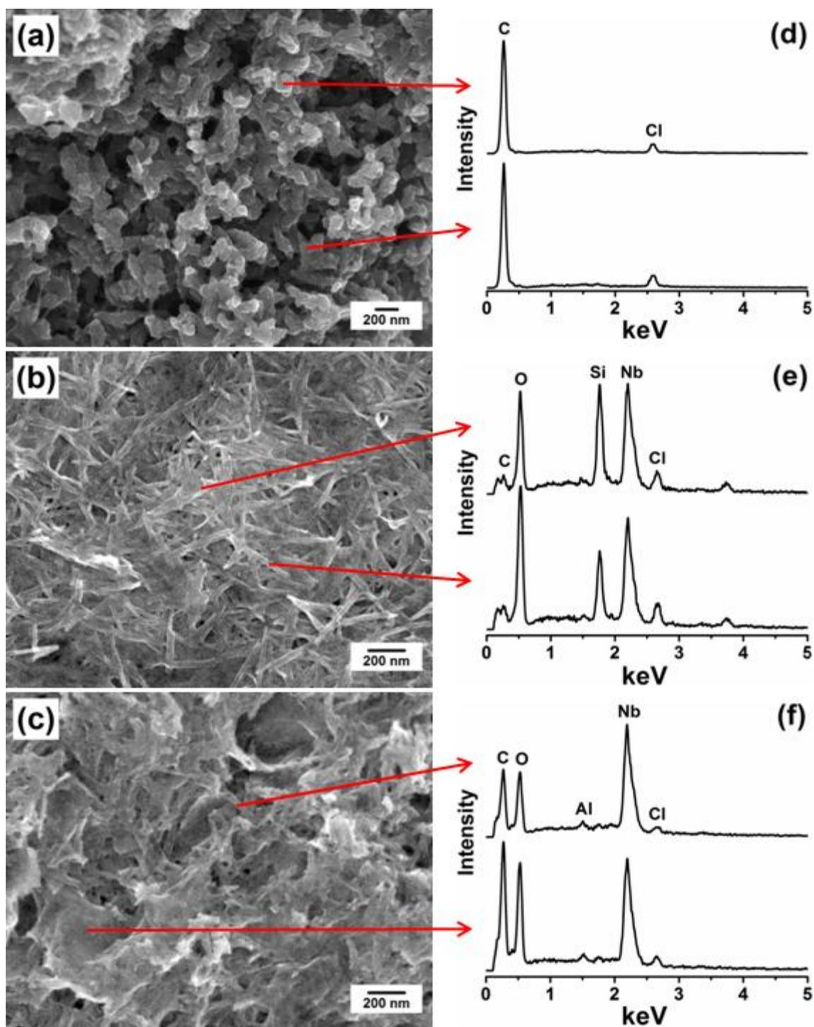
Figure 4. SEM images and EDX spectra of (a, d) PANI-ES, (b, e) NbONsc and (c, f) PNB(pH2.5). SEM image and EDX spectra of hybrid material PNB(pH0.1) are shown in Supporting Information (Figure S1).
