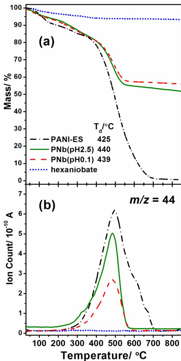
Figure 7. (a) TGA curves and (b) MS curves ( $m/z = 44$ ) of PANI-ES, hybrid materials PNb(pH2.5) and PNb(pH0.1), and hexaniobate.  $T_d$  are the on-set temperatures of irreversible decomposition of the PANI chains. Detailed information of TGA data are available in Supporting Information (figure S2).
