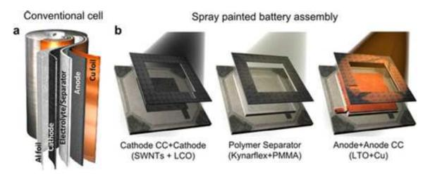
Figure 14 A schematic diagram illustrating the process for making paintable batteries. Reproduced from Ref. [161] with permission. Copyright 2012 Nature Publishing Group.
