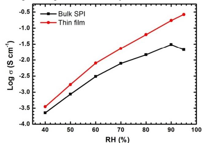
**Fig. 1** Relative-humidity-dependent proton conductivity plots for the pelletized bulk SPI and thin film.
