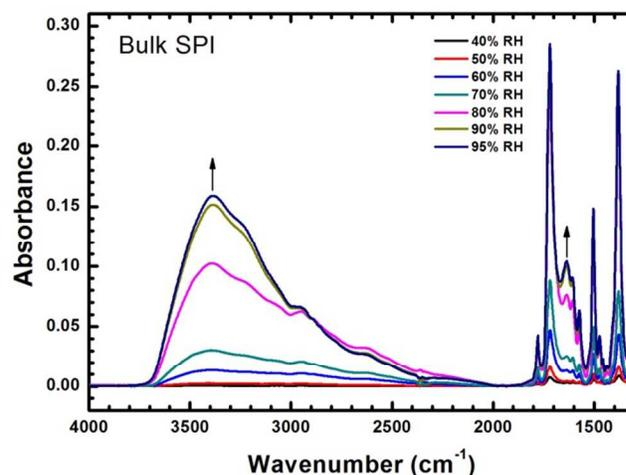
Fig. 8 An observation of the OH traces using FTIR-ATR spectra of the pelletized bulk SPI under various humidity conditions.
