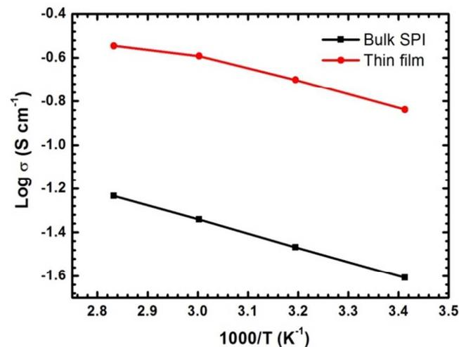
**Fig. 2** Temperature-dependent proton conductivity plots for the bulk and thin SPI film.
