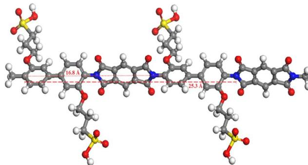
**Fig. 6** The DFT geometrical analysis performed for a rod-like SPI backbone and the obtained mean inter-distance values.
