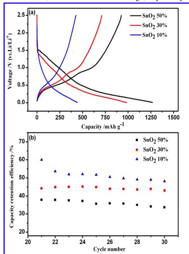
**Fig. 6** (a) Charge/discharge profiles and (b) capacity retention efficiency profiles of SnO<sub>2</sub>/C-10, SnO<sub>2</sub>/C-30 and SnO<sub>2</sub>/C-50
