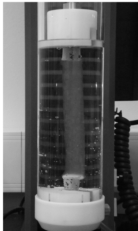
Fig. 3 Stress-strain measurement of a hydrogel under water.
