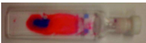
Figure 6. Colour change from blue to pink when sodium hydroxide was added to a solution of GEd polymers.
