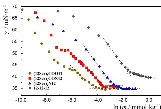
**Figure 2.** Surface tension versus  $\ln(\text{concentration})$  curves for the  $(12\text{Ser})_2\text{COO}12$ ,  $(12\text{Ser})_2\text{CON}12$  and  $(12\text{Ser})_2\text{N}12$  surfactants at  $25^\circ\text{C}$ . For comparison, the curve obtained for the conventional *bis*-quat gemini 12-12-12 is also shown.
