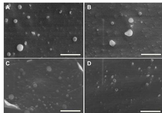
**Figure 8.** Cryo-SEM imaging for neat gemini and gemini/DOPE lipoplexes, at 5 mM and different charge ratios: A,  $(12\text{Ser})_2\text{COO}12$   $\text{CR}(+/-) = 12:1$ ; B,  $(12\text{Ser})_2\text{COO}12/\text{DOPE}$   $\text{CR}(+/-) = 4:1$ ; C,  $(12\text{Ser})_2\text{CON}12$   $\text{CR}(+/-) = 6:1$ ; and D,  $(12\text{Ser})_2\text{CON}12/\text{DOPE}$   $\text{CR}(+/-) = 4:1$ . Scale bars: 0.6  $\mu\text{m}$ . In all micrographs, vesicular structures are present.
