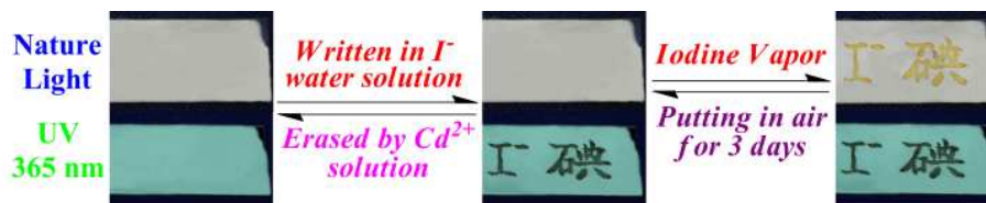
Fig. 4 Writing, erasing and coloration of a nature light invisible image on a CdG supramolecular gel film (obtained from 1% ethanol metallogel, CdG , G2 : \text{Cd}^{2+} = 1 : 1. Writing: written in \text{I}^- water solution; erasing: brushed by \text{Cd}^{2+} water solution; coloration: exposing the CdG film into the iodine vapour ca. 5 sec.) The photographs were taken at room temperature under room light and exposure to a 365-nm ultraviolet light.
