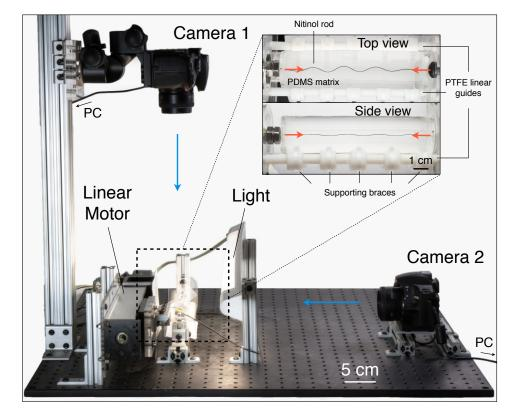
**Fig. 1** Experimental apparatus. A Nitinol rod is embedded within a cylindrical PDMS matrix (inside dashed frame). The sample is uniaxially compressed under displacement control. Two synchronized cameras placed on the top and side of the setup capture snapshots of the buckling of the rod (insets). The paired images are then sent to a computer for reconstruction of the configuration of the rod and further analyses.
