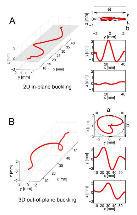
**Fig. 2** Experimental results. Buckled configurations of (A) Sample #1 and (B) Sample #2 acquired at  $\varepsilon = 3\%$  compressive strain. Both 3D and projected views (onto the *z*-*y*, *y*-*x* and *z*-*x*) are shown, clearly indicating that Sample #1 buckles into a 2D planar configurations, while Sample #2 buckles into a 3D coiled configuration. The dashed ellipse shown in the y-z view corresponds to the ellipse with minimum area that encloses the cross-sectional projection of the rod.
