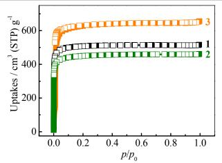
Fig. 2 N<sub>2</sub> adsorption (solid) and desorption (open) isotherms at 77 K for 1-3.
