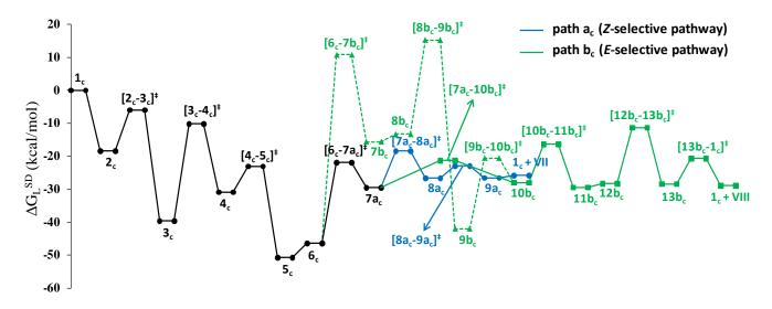
Figure 11. Overall reaction energy profile for the enamide formation using catalyst  $1_c$ . The dotted green line shows alternative vinylidene formation steps from vinyl intermediate  $6_c$ .
