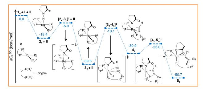
**Figure 6.** Energy profile for the oxidative addition and hexyne insertion steps for catalytic system  $\mathbf{1}_{c}$ . Ball and stick structures of the computed species with labeling of atoms, geometrical parameters and energy profiles are collected in Figures S18-S19.
