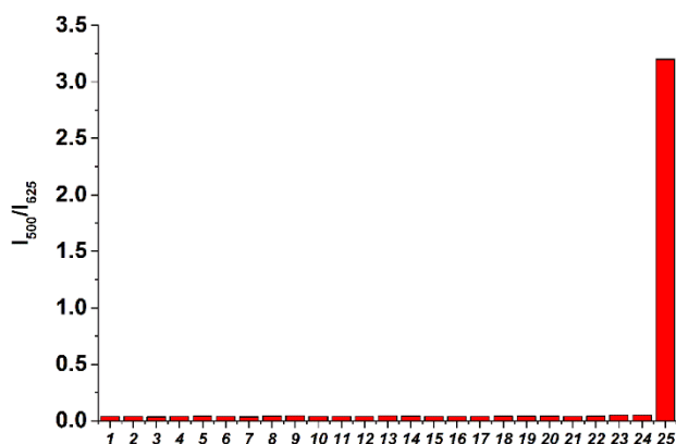
Fig. 3. Fluorescence intensity ratios ( I_{500}/I_{625} ) responses of probe TR-H 2 S (2 \mu M) to representative species in PBS buffer (pH = 7.4, 2% DMSO, 1 mg/mL HSA). (1) Free, (2) t BuOOH (200 \mu M), (3) NO (200 \mu M), (4) (5) H 2 O 2 (200 \mu M), (6) KO 2 , (200 \mu M), (7) Lys (200 \mu M), (8) HOCl (100 \mu M), (9) NH 3 ·H 2 O (200 \mu M), (10) HO·(200 \mu M), (11) NO 2 - (200 \mu M), (12) NO 3 - (200 \mu M), (13) Glu (200 \mu M), (14) N 3 - (200 \mu M), (15) CN - (200 \mu M), (16) K + (5 mM), (17) Na + (5 mM), (18) Ca 2+ (1 mM), (19) Zn 2+ (1 mM), (20) Mg 2+ (500 \mu M), (21) S 2 O 3 2- (200 \mu M); (22) SCN - (100 \mu M); (23) SO 4 2- (500 \mu M); (24) Cys (1 mM), (25) H 2 S (100 \mu M).
