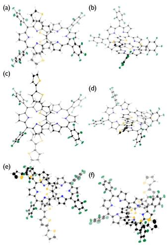
Fig. 2. X-Ray crystal structures of (a,b) **T2**, (c,d) **T3**, and (e,f) **T4**. Solvent molecules are omitted for clarity. The thermal ellipsoids are scaled to 30% probability level. One of the two molecules in the unit cell is shown for **T2** and **T4**.
