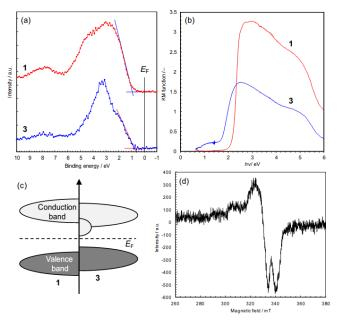
Figure 7 Spectroscopic data of the frontier orbitals in 1 and 3. (a) XPS data of valence bands. The valence band maxima were obtained by extrapolation of the onset linear parts: 1.0 eV for 1 and 0.8 eV for 3. (b) Kubelka-Munk functions obtained by diffuse reflectance spectroscopy. (c) Schematic illustration of the positions of the frontier orbitals. (d) X-band ESR spectra for Cu(II) ions in 3.
