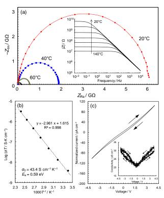
**Figure 3** AC Impedance analyses. (a) Complex-plane impedance data for a pellet of **3** (red: 20°C; blue: 40°C; green: 60°C; and black: 80°C). The inset shows  $\log |Z|$  vs log frequency plots. (b) Arrhenius plot of the electronic conductivity. (c) Current-voltage characteristics measured by cyclic voltammetry scanned at 10 mV s<sup>-1</sup> at 25°C.
