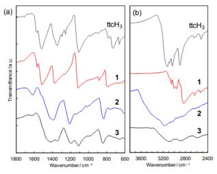
Figure 4 FTIR spectra of 1, 2 and 3 compared with pure trithiocyanuric acid. (a) 600–1800 cm<sup>-1</sup>. (b) 2400–3800 cm<sup>-1</sup>.
