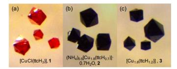
Figure 2 Photos of (a) 1 CuCl(ttcH $_3$ ) crystals, (b) 2 – i.e. 1 treated in aqueous ammonia for 2 days, and (c) 3 – i.e. 2 dried at 130°C under vacuum. The large monoliths are about 100  $\mu$ m across.
