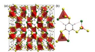
**Figure 1** Crystal structure of [CuCl(ttcH<sub>3</sub>)].<sup>13</sup> (a) 2×2×2 cells. (b) Connectivity of CuClS<sub>3</sub> tetrahedral with the thioketone form of trithiocyanuric acid molecules (red: Cu, green: Cl, yellow: S, blue: N, brown: C, and white: H). Dotted lines show hydrogen bonding.
