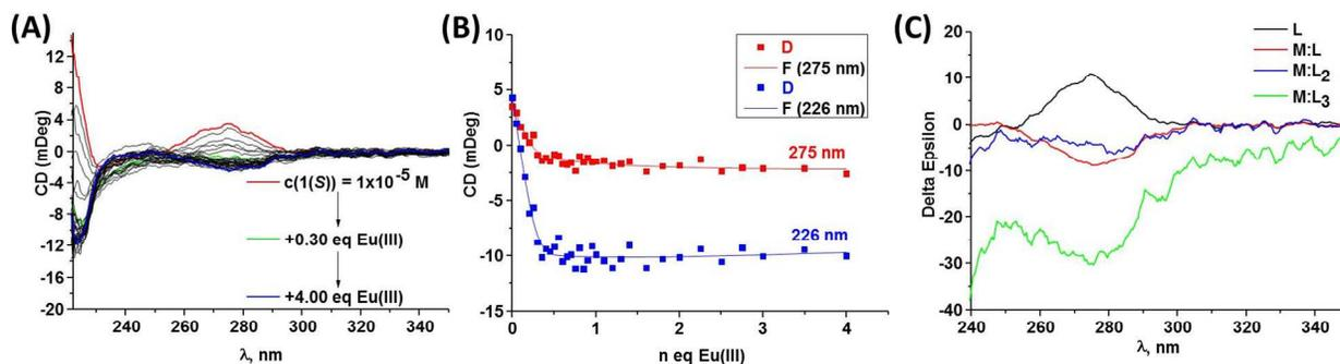
Figure 8. (A) Changes in CD spectra of **1(S)** (—) ( $c = 1 \times 10^{-5}$  M) upon addition of Eu(CF<sub>3</sub>SO<sub>3</sub>)<sub>3</sub>, (B) experimental binding isotherms representing the changes in the CD bands upon gradual Eu(CF<sub>3</sub>SO<sub>3</sub>)<sub>3</sub> addition in CH<sub>3</sub>CN (25 °C, 0.05 M (C<sub>2</sub>H<sub>5</sub>)<sub>4</sub>NCl) and (C) recalculated CD spectra obtained with SPECIFIT<sup>®</sup>.
