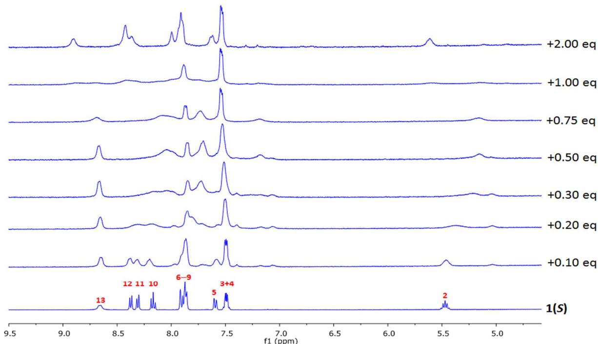
Figure 6. The changes in the  $^1\text{H}$  NMR spectra (400 MHz) of **1(S)** ( $c = 4.26 \times 10^{-4}$  M) upon gradual addition of  $\text{La}(\text{CF}_3\text{SO}_3)_3$  in  $\text{CD}_3\text{CN}$ .
