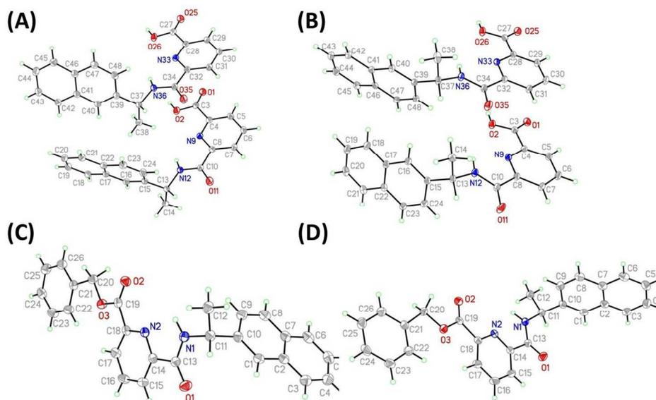
**Figure 2.** Molecular structures of (A) **1(R)** and (B) **1(S)** showing both independent molecules in the asymmetric unit, (C) **4(R)** and (D) **4(S)** (thermal displacement 50%).
