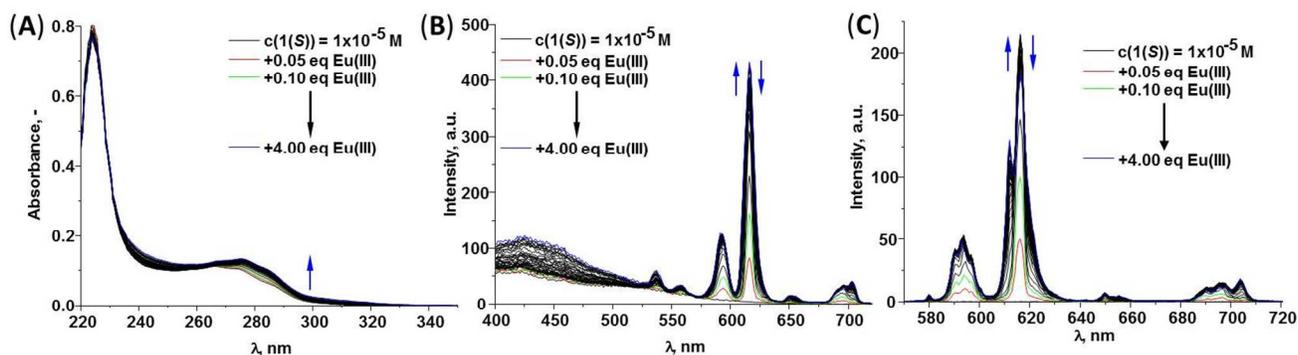
**Figure 4.** The changes in the (A) absorption, (B) fluorescence and (C) Eu(III)-centred emission spectra of **1(S)** ( $c = 1 \times 10^{-5}$  M) upon addition of  $\text{Eu}(\text{CF}_3\text{SO}_3)_3$  in  $\text{CH}_3\text{CN}$  (25 °C, 0.05 M  $(\text{C}_2\text{H}_5)_4\text{NCl}$ ).
