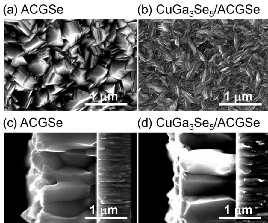
**Fig. 6** Top and cross-sectional SEM images of ACGSe (a), (c), and  $\text{CuGa}_3\text{Se}_5/\text{ACGSe}$  with  $\text{CuGa}_3\text{Se}_5$  deposited for 15 min (b), (d).
