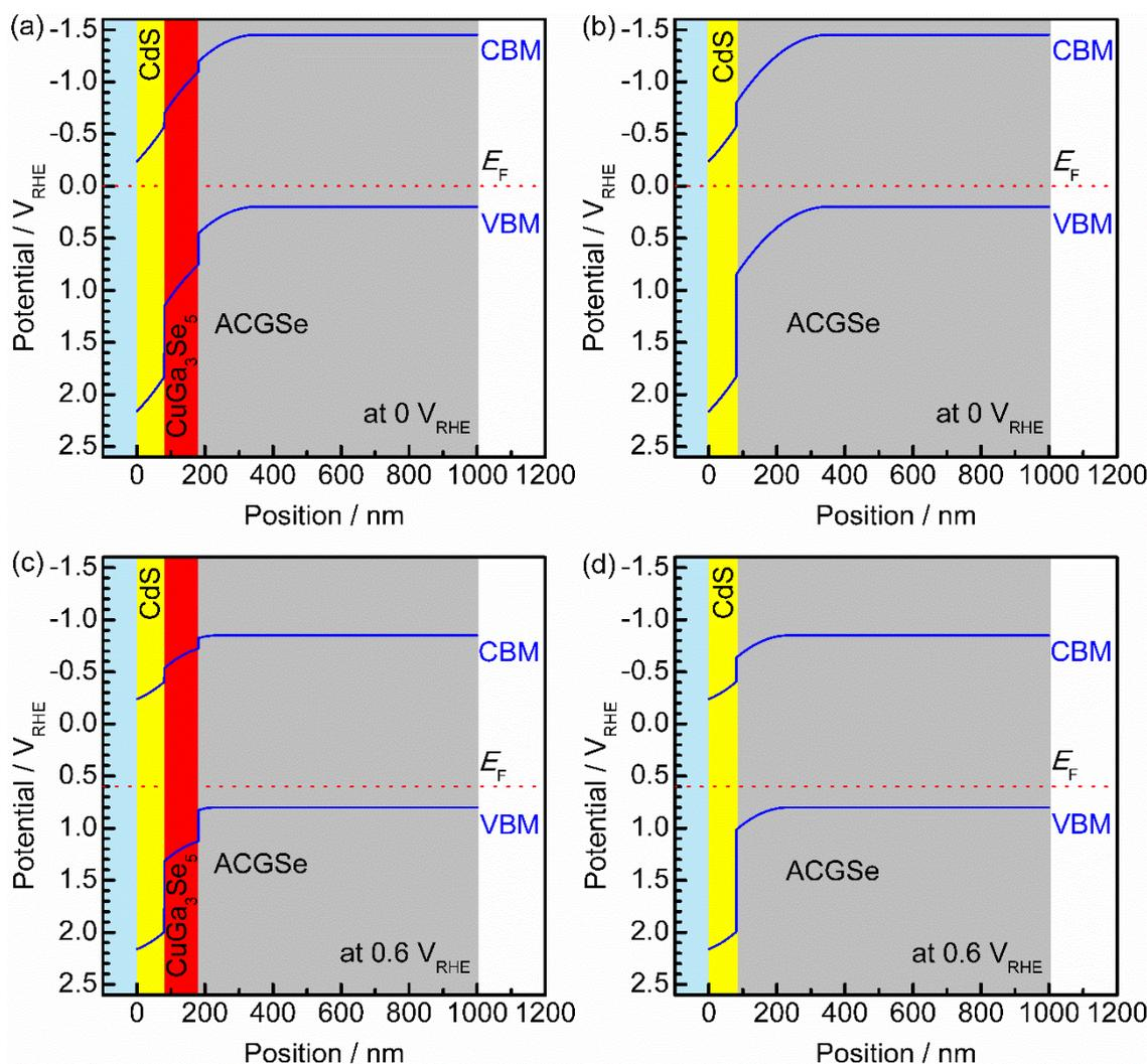
**Fig. 8** Calculated band alignment near solid-liquid interface for CdS/CuGa<sub>3</sub>Se<sub>5</sub>/ACGSe with CuGa<sub>3</sub>Se<sub>5</sub> deposited for 15 min, and Pt/CdS/ACGSe at an applied potential of 0 V<sub>RHE</sub> (a), (b), and 0.6 V<sub>RHE</sub> (c), (d). VBM, CBM and E<sub>F</sub> denote the valence-band maximum, conduction-band minimum, and Fermi energy, respectively.
