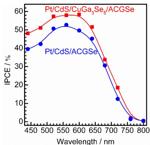
**Fig. 2** Wavelength dependence of IPCE spectra for Pt/CdS/CuGa<sub>3</sub>Se<sub>5</sub>/ACGSe with CuGa<sub>3</sub>Se<sub>5</sub> deposited for 15 min, and Pt/CdS/ACGSe measured at an applied potential of 0 V<sub>RHE</sub>. The IPCE was measured in 0.1 M Na<sub>2</sub>HPO<sub>4</sub> (adjusted to pH 10 by addition of NaOH) under monochromatic light from a 300 W Xe lamp equipped with band-pass filters and an optical fiber.
