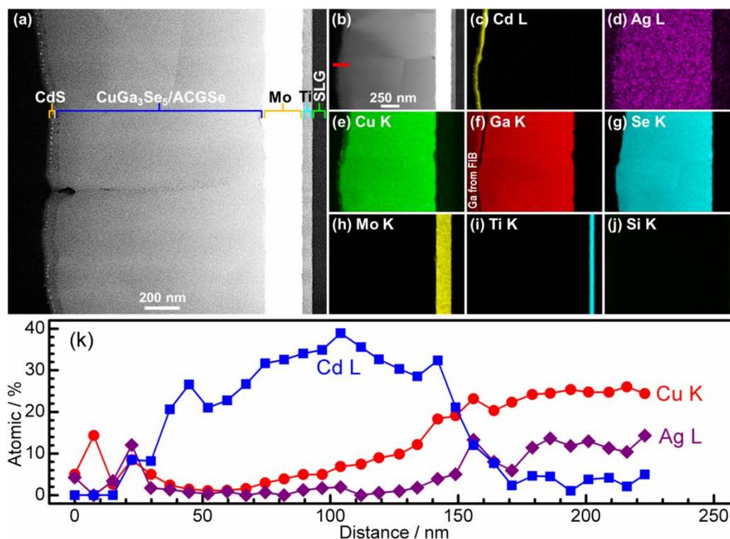
**Fig. 7** Cross-sectional TEM images of CdS/CuGa<sub>3</sub>Se<sub>5</sub>/ACGSe sample with CuGa<sub>3</sub>Se<sub>5</sub> deposited for 15 min (a), (b); EDX elemental maps for Cd (c), Ag (d), Cu (e), Ga (f), Se (g), Mo (h), Ti (i), Si (j); and line profiles for Cd, Cu and Ag across the CdS and CuGa<sub>3</sub>Se<sub>5</sub>/ACGSe interfaces (k). The red line in Fig. 4(b) indicates where the linear profile was measured. The sample was sliced using a Ga focused ion beam (FIB).
