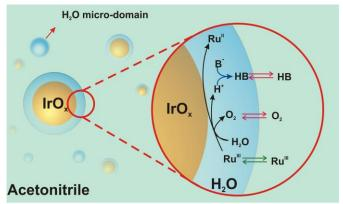
**Scheme 1.** Proposed formation of reactive water overlayers on  $IrO_2$  nanoparticles.  $Ru^{III} = [Ru^{III}(bpy)_3]^{3+}$ ,  $Ru^{II} = [Ru^{II}(bpy)_3]^{2+}$  and  $B^-$  = proton acceptor species (in the absence of any additional basic specie  $B = H_2O$ )
