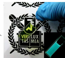
Fig. 1 Chemical structure of cyanostilbene-containing gelator molecule, 1 (PyG) and photo image of its transparent gel in cyclohexane (1 wt%) under room light. Inset shows the fluorescence photo image of the gel under UV light.
